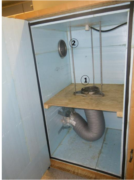
Figure 5.3 Wooden cabinet and drying air inlet and outlet tubes numbered as (1) and (2) respectively
