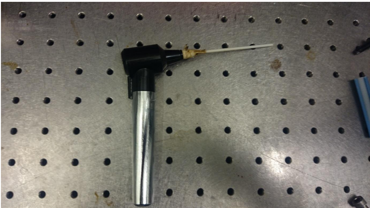
Figure 3.6 Picture of the handheld mixer used to mix the to liquids in these experiments
