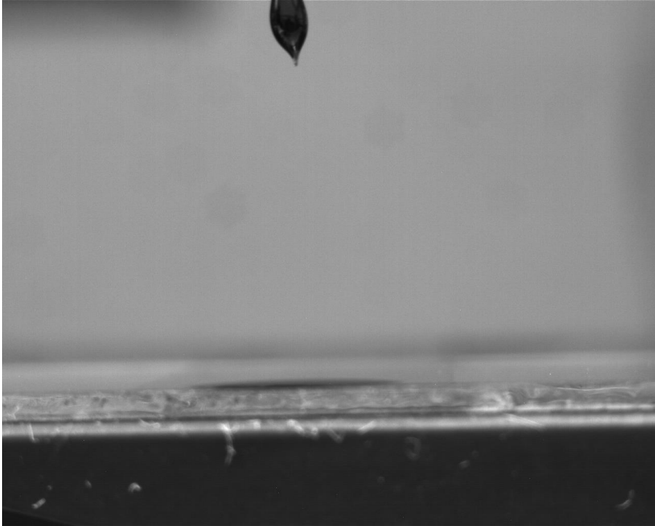
Figure 5.33 Picture of crude oil on the ITO 30 surface.
