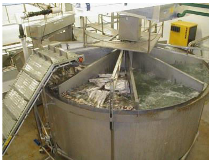
Figure 32: A cylindrical thawing tank as build by (Melbu Systems AS, 2017)
