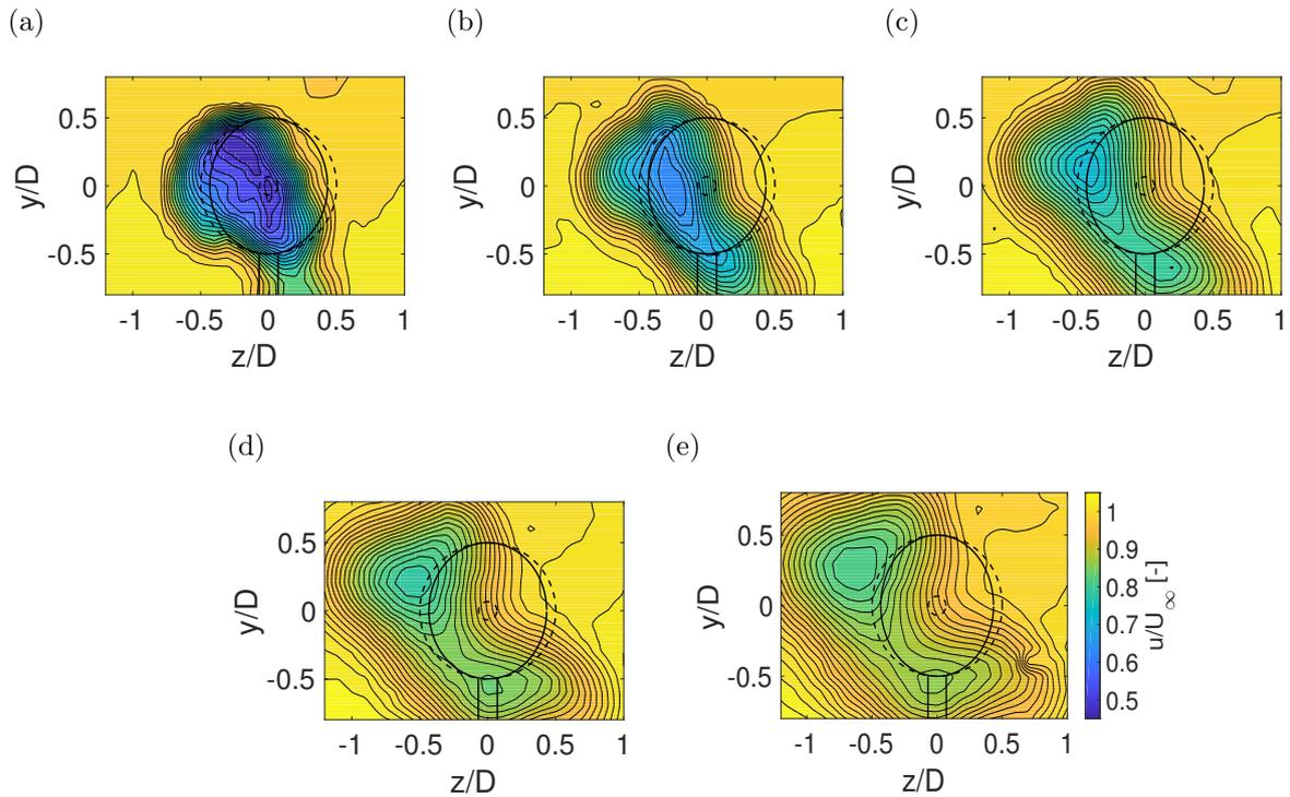
Figure 5: Normalized velocity distribution of the cross-section of the wake when the turbine in a  $30^\circ$  of yaw. The distances shown are (a) 3D, (b) 6D, (c) 9D, (d) 12D, and (e) 15D downstream from the turbine. The solid line illustrates the outline of the yawed turbine, while the dotted line illustrates the outline of an imaginary non-yawed turbine.
