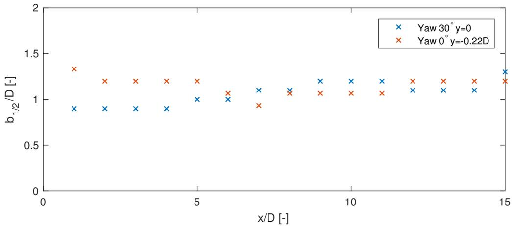
Figure 8: The normalized half-width development of the wake with the turbine in both non-yawed condition (orange) and yaw angle of  $30^\circ$  (blue).
