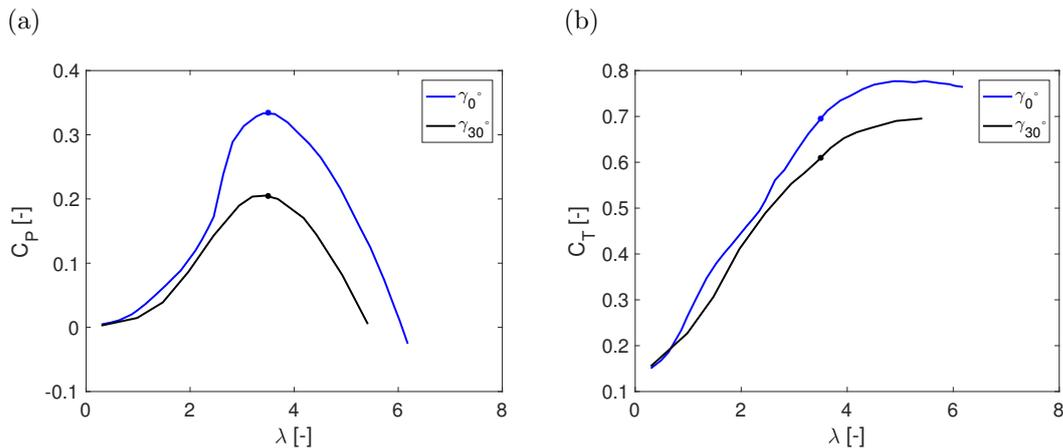
Figure 2: The turbine performance is presented by the curves of (a) the coefficient of power,  $C_P$ , and (b) the coefficient of thrust,  $C_T$ , both with respect to TSR. The optimal TSR ( $\lambda = 3.5$ ), which was used in the experiments, is indicated on the curve by an asterisk (\*).
