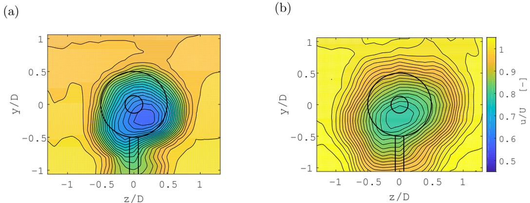
Figure 3: Normalized velocity distribution of the cross section of the wake in non-yawed condition, measured at distances (a) 6D and (b) 12 D downstream of the turbine. The black solid lines illustrate the outline of the non-yawed turbine.
