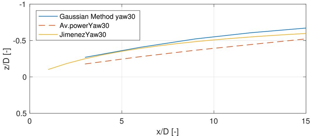
Figure 9: Center wake trajectory estimated by the Gaussian Method (blue), the Available Power method (orange) and the analytical model by Jimenez (yellow). The evaluation is performed with optimal TSR and yaw angle of  $\gamma = 30^\circ$ .
