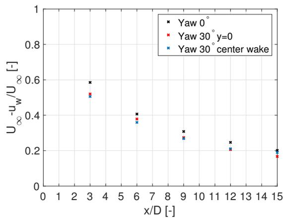
Figure 6: The maximum normalized velocity deficit of the wake at several distances downstream. The values from the turbine in non-yawed condition (black),  $\gamma = 30^\circ$  with measurements at  $y = 0$  (red) and  $\gamma = 30^\circ$  with velocities in the wake center (blue) are shown.
