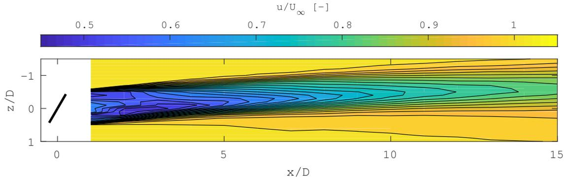
Figure 4: Normalized velocity distribution of the wake with the turbine at yaw  $30^\circ$ . The wake is seen from above and the solid black line illustrate the yawed turbine.
