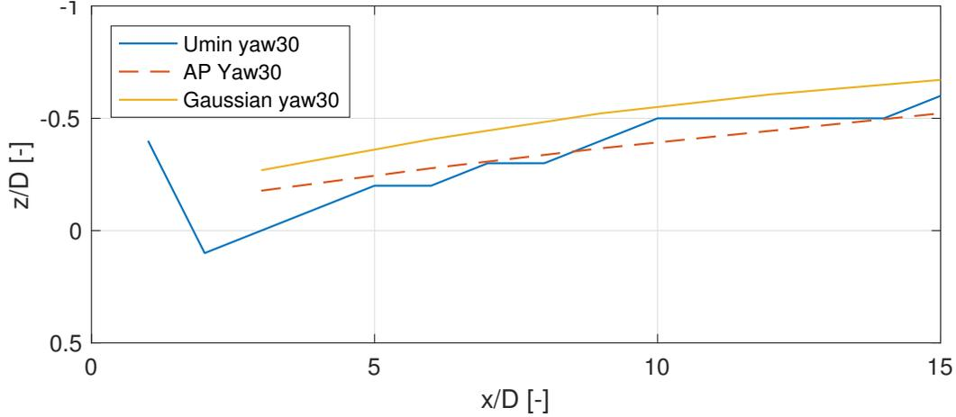
Figure 7: The wake center line trajectory is presented by using three different methods; the  $U_{min}$  Method (blue line), the *Available Power Method* (orange dotted line), and the *Gaussian Fit Method* (yellow line).
