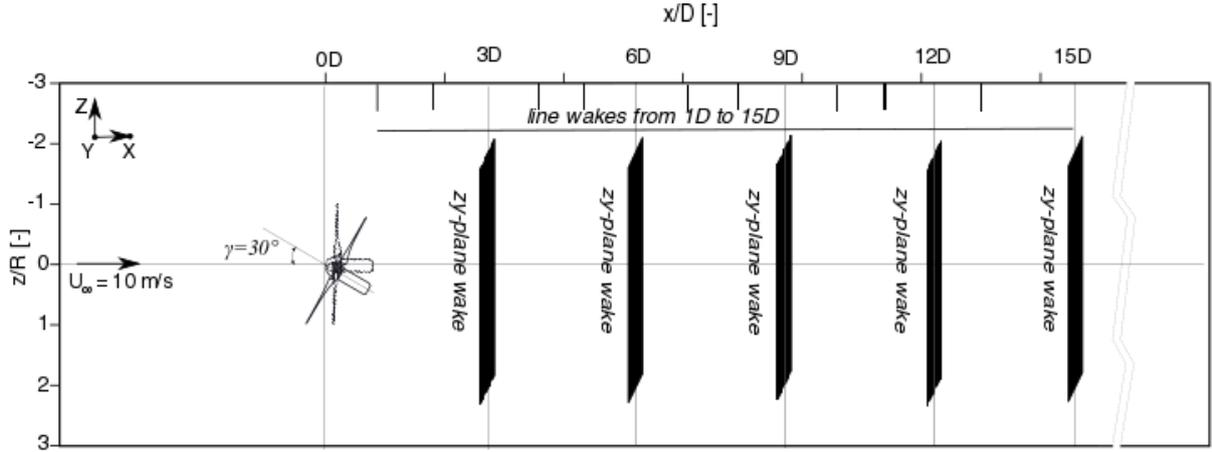
Figure 1: A simple sketch of the composition of the experiments performed in the wind tunnel. The yaw angle is defined positive in the clockwise direction.
