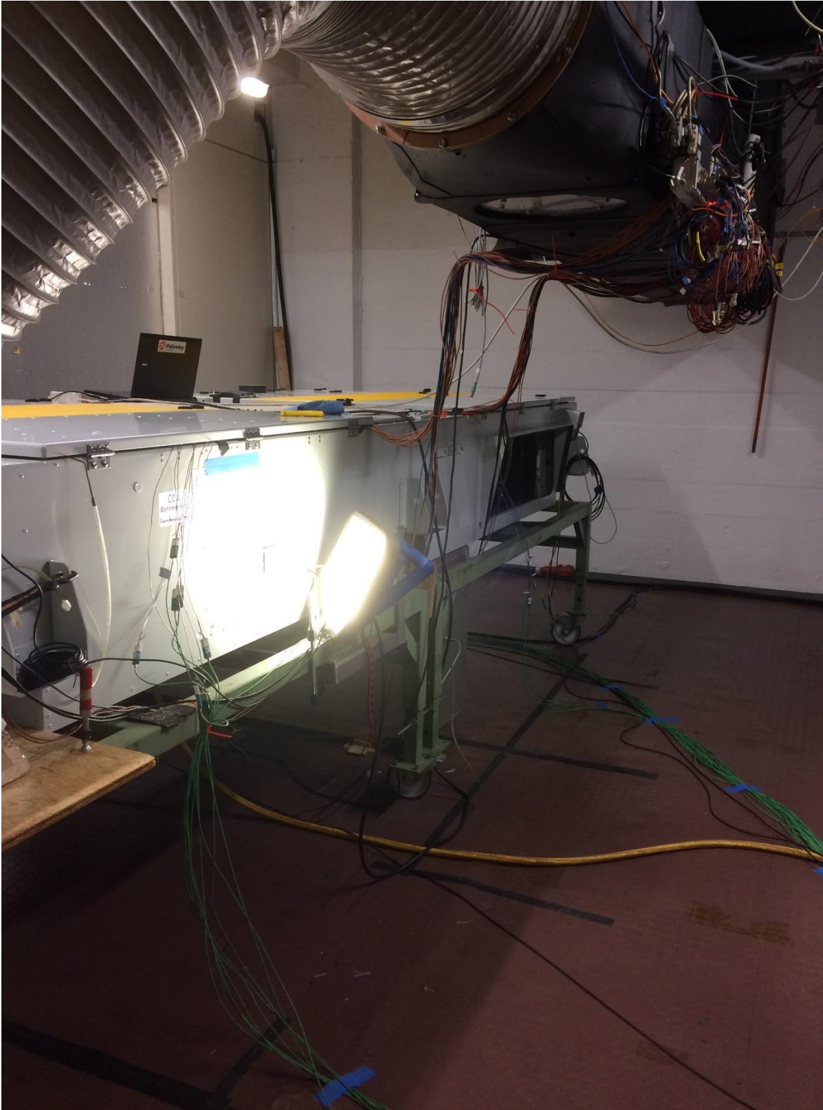
Pilot R744 HVAC unit casing inside the FTL test chamber
