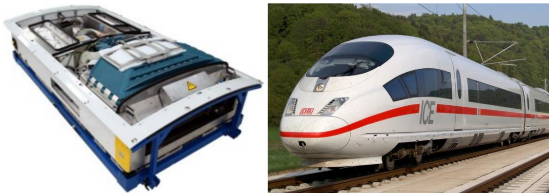
Figure 2.6: Air cycle AC onboard DB intercity ICE-3 trains. Right: DB ICE-3 [Deutsche Bahn], left: air cycle AC unit from Liebherr for the ICE 3.1 Re-Design program (Liebherr).
