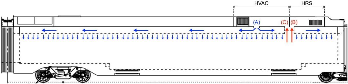
Figure 3.7: Distribution of ventilation air onboard the NSB Stadler FLIRT. Where the blue arrows represent flow of fresh air, the red arrows represent flow of extract air, (A) is the supply air outlet of the HVAC unit connected to the supply air distribution ductwork, (B) is the extract air inlet of the HRS, and (C) is the return air inlet for the AHU.
