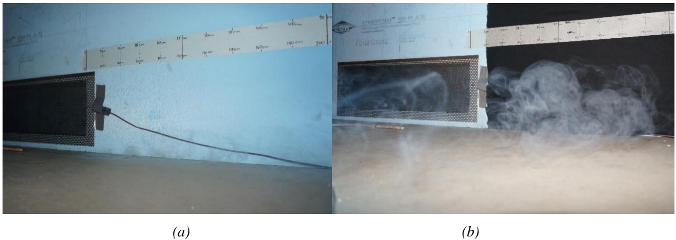
Figure 5.7 Smoke visualization from supply diffuser. No floor heating. (a) Smoke move close to floor, along the back internal wall. (b) Smoke move toward the south-east work stations, mixing more in height.
