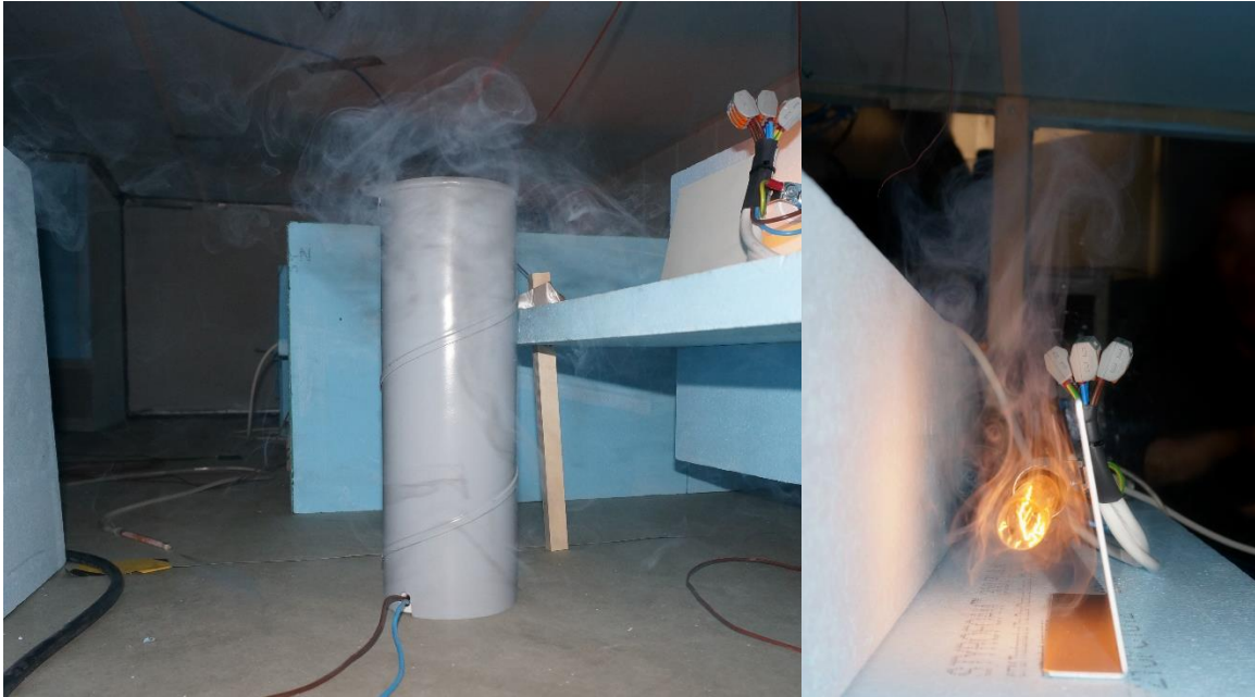
Figure 5.8 Smoke visualization of thermal plume from simulated person (left) and computer (right).
