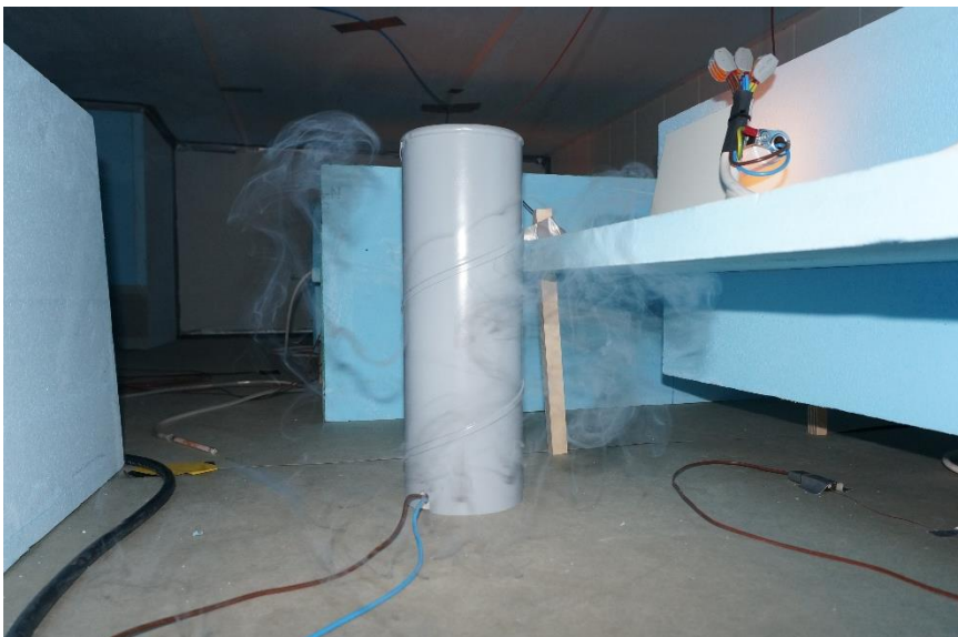
Figure 5.9 Smoke hindered by the desk divider in the east corner. The desk divider can be seen both underneath and above the desk.
