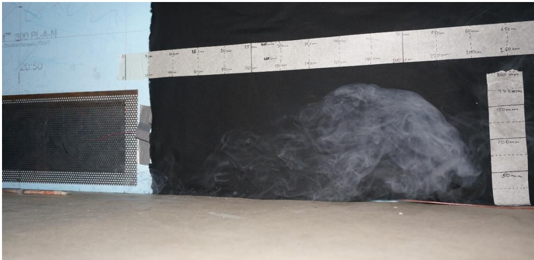
Figure 5.6 Smoke visualization of supply air diffuser. Smoke in eastern direction. No floor heating. The diffuser in the picture is the one used for velocity mapping, circled in red in Figure 4.2.
