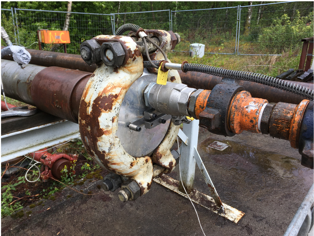
Figure B.5: Photograph showing the ball valve without the rotating disc mounted and the slit sealed off
