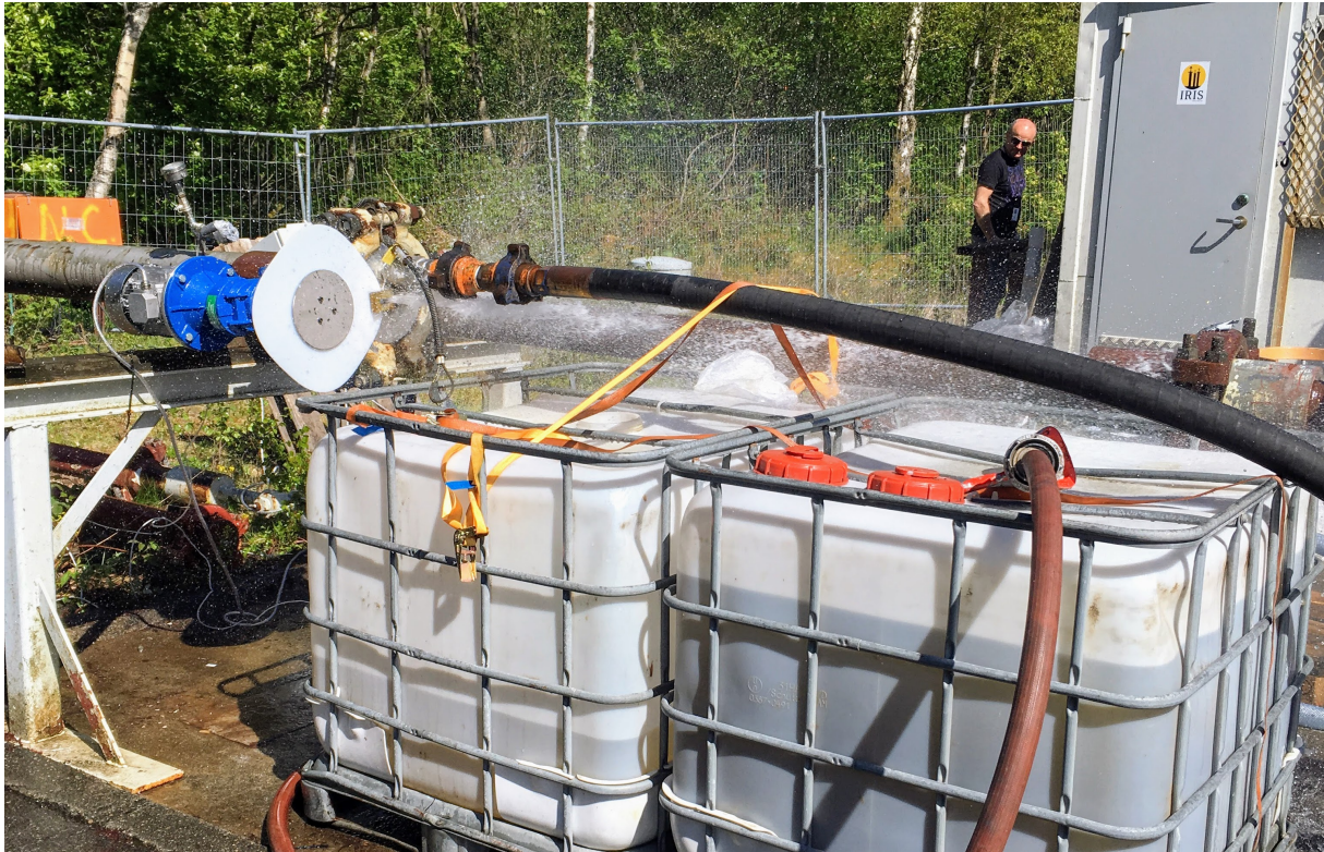
Figure B.6: Photograph of the rotating disc during operation
