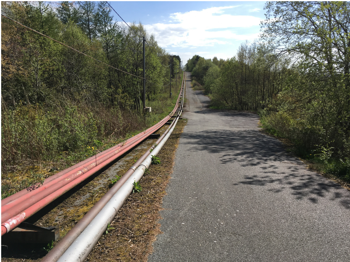
Figure B.4: Photograph from test facility showing the length of the pipes
