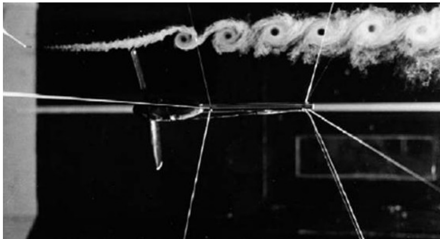
Figure 2.5: Tip vortices visualized using smoke [7]
