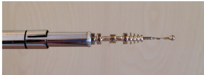
Figure (5.1): Transducer from AirDistSys 5000. Picture by Solveig Blandkjenn
