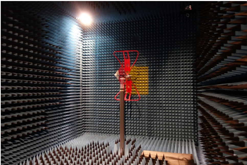
Figure 5.4: The receiving antenna in the anechoic chamber oriented to receive the vertical field component
