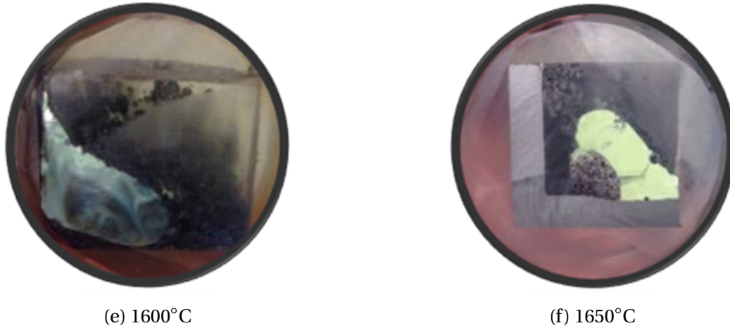
Figure 4.23: Image a) shows the interior of crucible heated to 1650°C where foaming can be confirmed by the small metal particles covering the inside of the crucible surface. Image b)-f) shows samples after mounting in epoxy displaying bottom surface of the slag.
