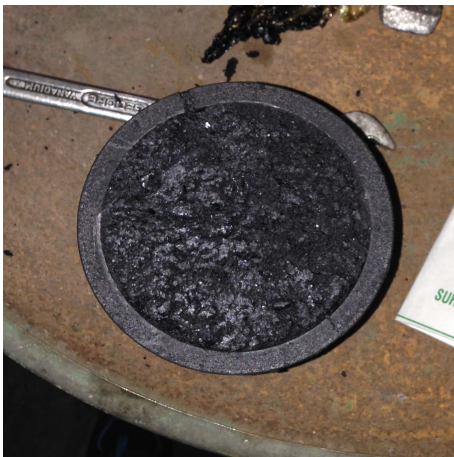
(c) Graphite crucible filled with clay
