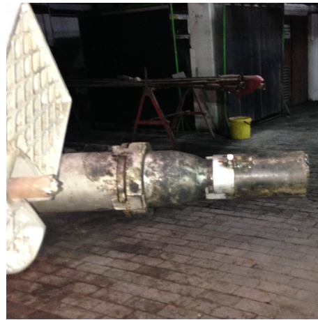
(b) Metal cast connected to mudgun
