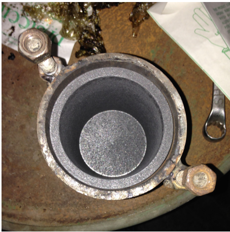
(a) Graphite crucible inside metal cast
