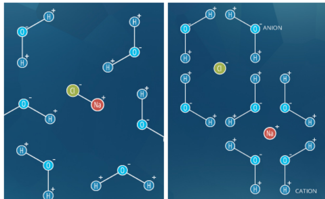
Figure 2.3: When salts are dissolved in water they split into an anion and a cation. These ions make up the basis of conductivity in water [13].
