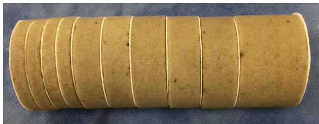
Figure 4.6: Assembled core consisting of all samples with filter paper between each core piece. The picture is taken prior to toluene-flooding core after the cores had been saturated with high-salinity water. The left side was inserted near the inlet.
