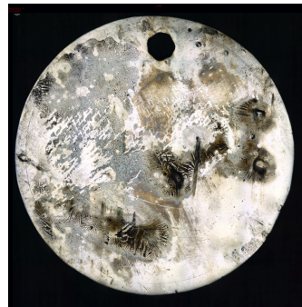
(i) Sample T2t5-2 with a CPT below 40°C.
