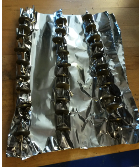
Figure 3.2.1: The tray made of stainless steel, with samples placed in their rooms, used when heat treating the samples.
