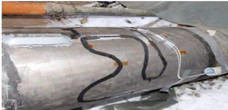
Figure 21: Distributed fiber optic sensor along a pipeline (azosensors.com)
