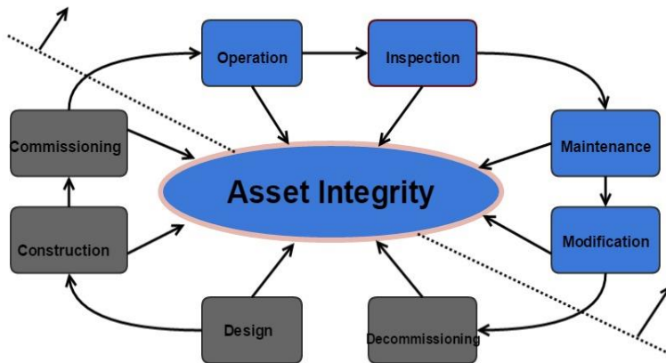
Figure 6: Elements that have impact on the integrity of an asset over its entire life-cycle. Source: HSE (2006) but adopted from (Hassan and Khan, 2011).
