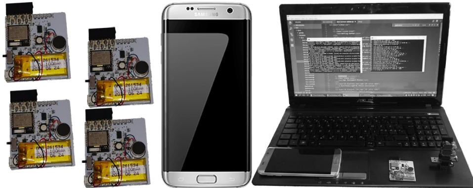
Figure B-1, What you need for IoT prototyping with the TILES toolkit
