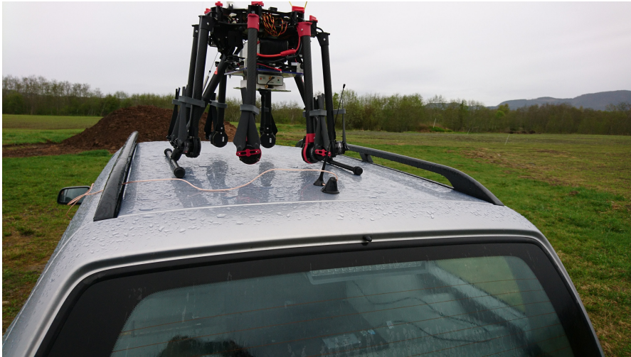
Figure 5.8: Placement of the magnetic base antenna close to existing antenna on the vehicle, which is disassembled under the measurements. The home position is also shown to be at the middle of the vehicle roof.
