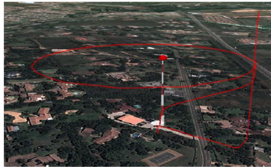
(b) Flight path of the measurements around the antenna illustrated with a geographical representation.
