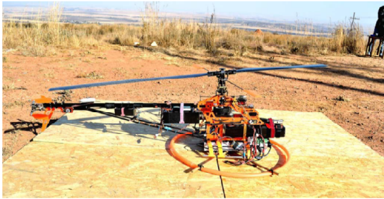
(a) Miniature helicopter used in the research with measurement system mounted under the landing skids.
