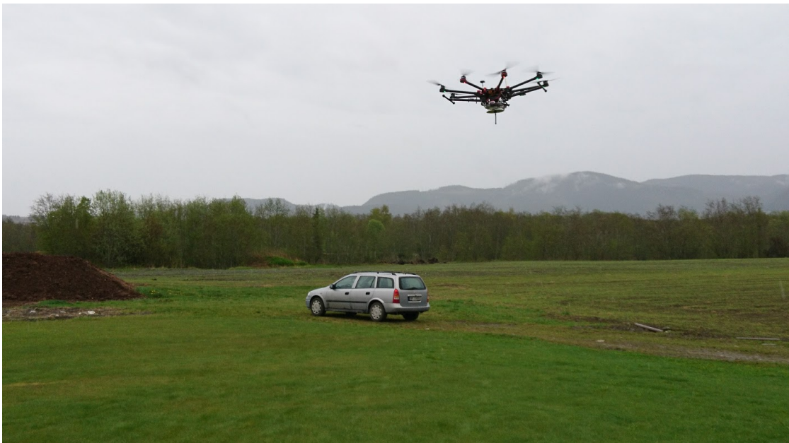
Figure 5.5: Picture of the multicopter when measuring the magnetic base roof antenna.
