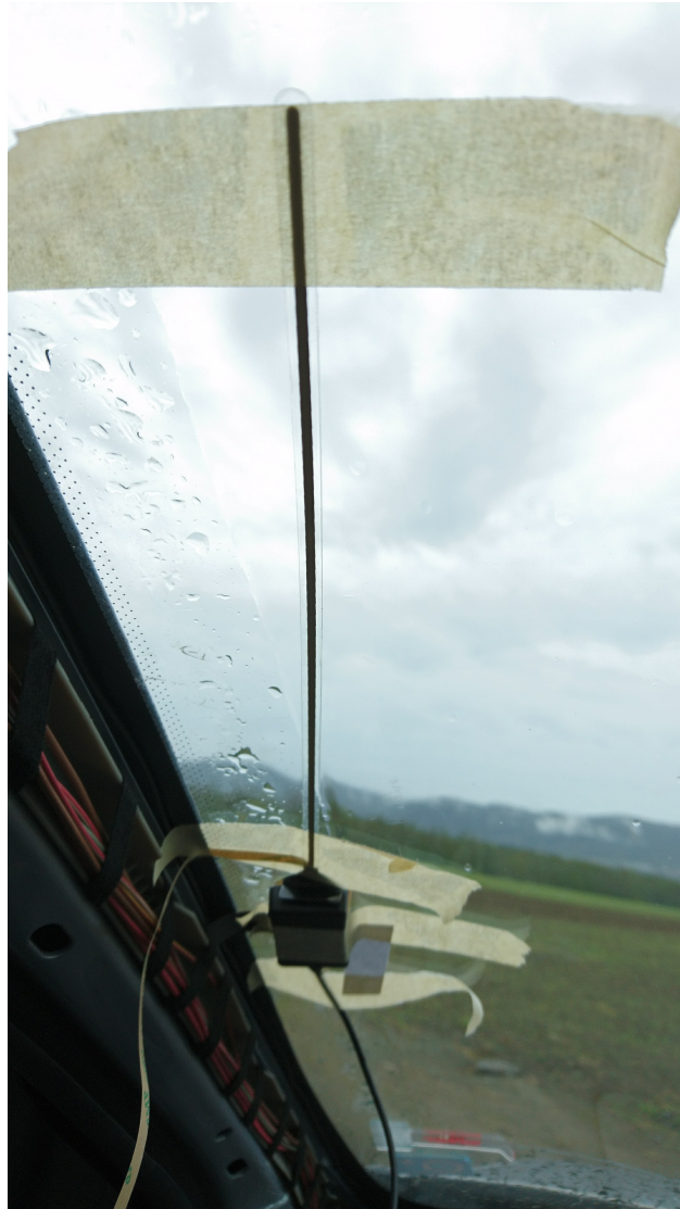
Figure 5.15: Placement of the windshield antenna on at the left side of the vehicle windshield grounded to the chassis at the window pillar and positioned from 20 cm to 35 cm down from the roof with an angle of about 60^\circ from the altitude axis.
