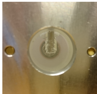
(b) View of counter electrode inside the cell during charging
