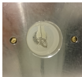
(b) View of platinum wire counter electrode inside cell
