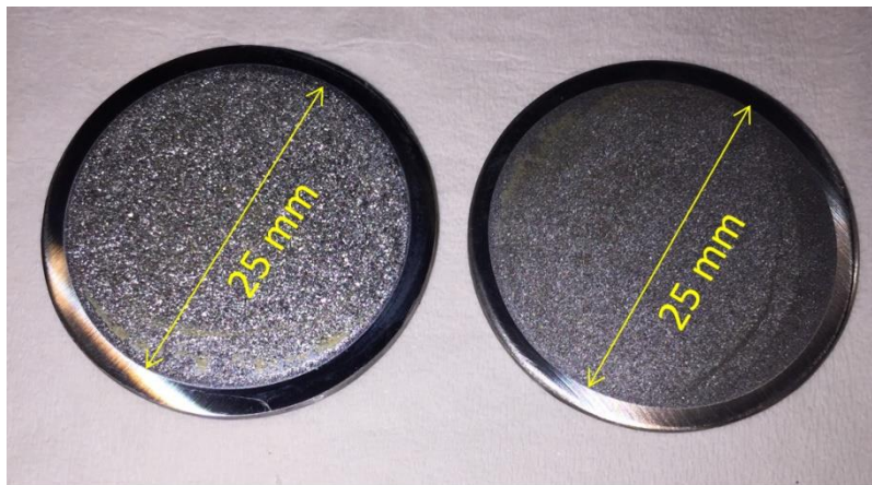
Figure 45 Picture of the specimens after the polarization curves were recorded. 0 Ni to the left, and 3 Ni to the right. Both the diameters of the corroded areas were 25 mm.
