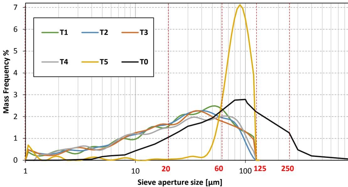
Figure 4-10: The mass frequency of the different TBM materials. Minor variation in the frequency of the 4 TBM spoils. The processed 0/8 mm follo line aggregate(T5) do show high occurrence between 60-125 μm. This can be explained by the reduction of fines with the cyclone placed at Åsland.
