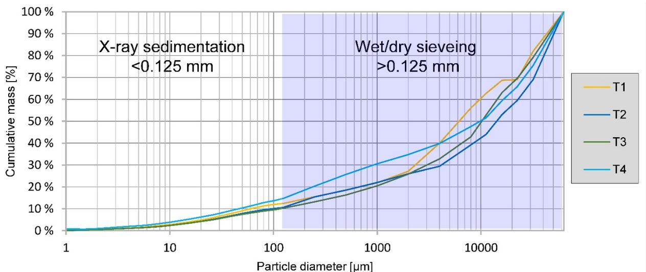
Figure 5-1: The PSDs produced can be combined. The X-ray sedimentation PSDs are not easy to differentiate at this scale.
