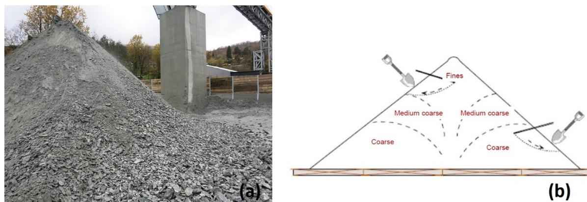
Figure 3-3: (a): Showing stock pile at Ulriken tunnel project, sample 2 was taken from this pile. (b): the normal segregation generated when piles are created from conveyer belts.
