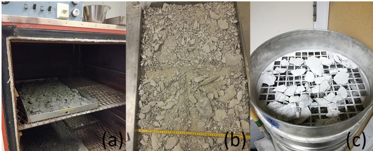
Figure 3-4: (a) Drying TBM spoil at 105 °C. (b) Reducing sample by quartering for further dry sieving. (c) Dry sieving of TBM spoil.
