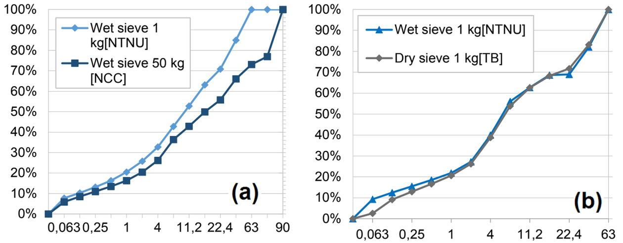
Figure 4-6: Proving differences in the use of wet and dry sieving technique and the amount used (kg) Left: T3, Right: T1.
