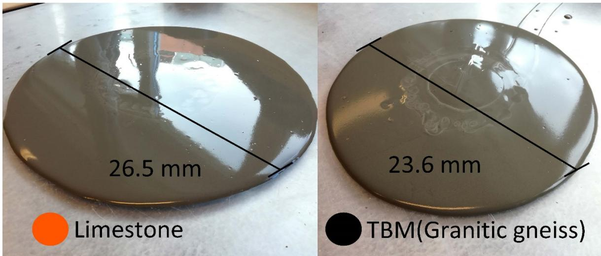
Figure 4-13: Comparing the most similar mini-slump values between the limestone and the TBM filler (T0 vs T1).
