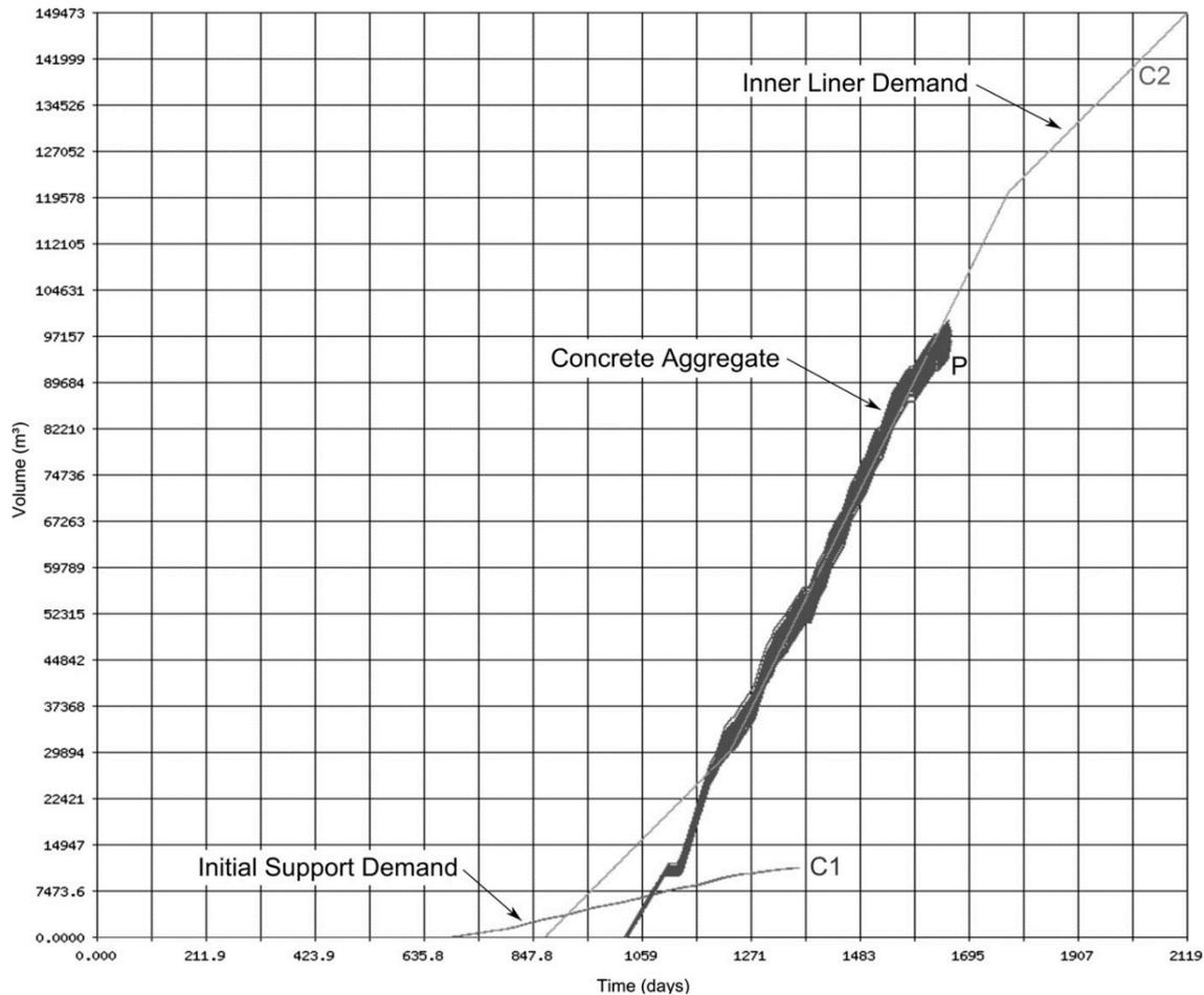
Figure 2-45: Concrete aggregate consumption through a four-year tunnel project versus the self-produced concrete aggregate. Grey area represents 100 different simulations which are based on uncertainties as evading geological conditions [23]. Self-supply of concrete aggregates is obtained 424 days after concrete consumption starts.
