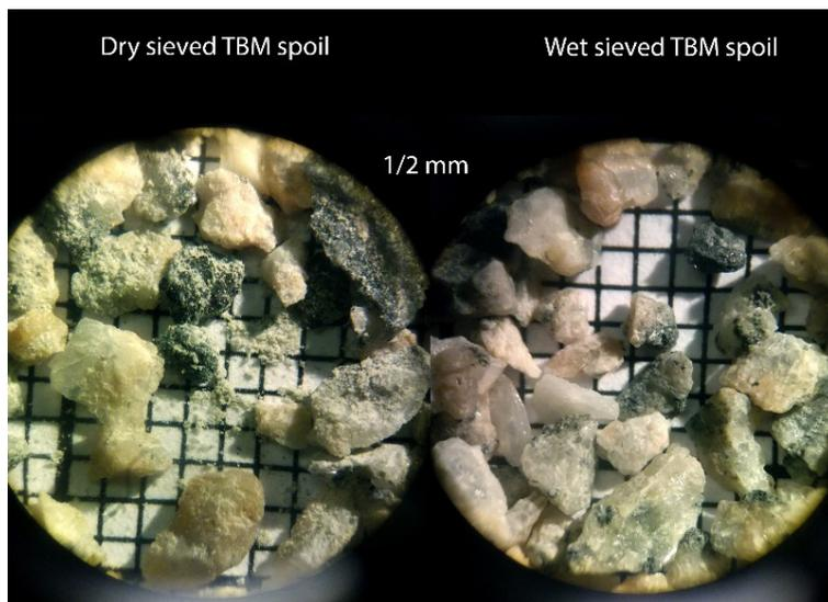
Figure 4-5: Fines have a cohesive binding to particles which stick to the dry sieved spoil. Light scraping on the dry sieved 1/2 mm fraction and finer particles fell off. Squares are 1 mm.
