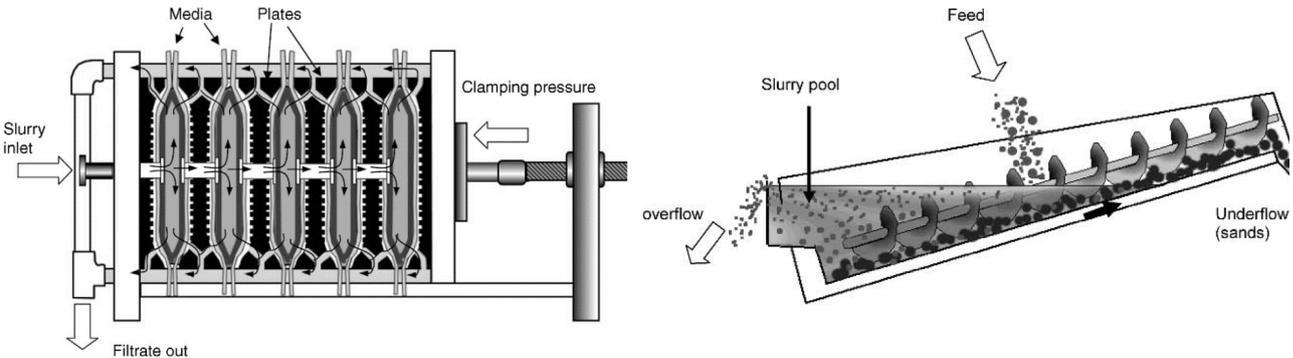
Figure 2-15: Left: dewatering of mud water with filter press (VPA) for removal of fines [62]. Right: Dewatering of coarser particles with a bottom spiral classifier [62].
