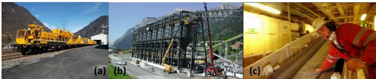
Figure 2-36: (a) The concrete batching plant train[92]. (b) Aggregate silos for the concrete train at Amsteg, (c) Inspecting aggregate quality at Amsteg aggregate plant [93].
