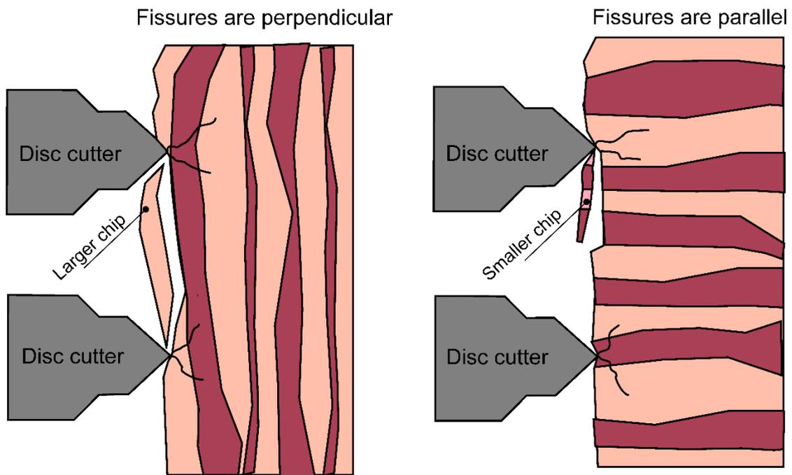
Figure 2-4: Anisotropy in relation to the cutter face angle will impact the spoil properties. Tunnelling perpendicular to the direction of fissure direction tends to generate larger and more elongated chips [28].
