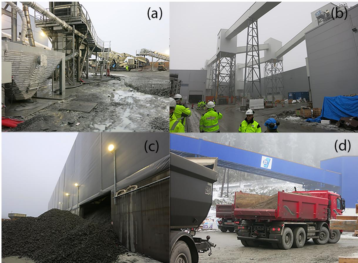
Figure 3-2: (a) Processing facility at the follo line project, dewatering cyclone can be seen in front, in the back a mobile screener combined with a cone crusher. (b) Conveyer system, concrete batching plants and segment production. (c) High quality spoil, this would be transported by wheel loader into the scalping screen and material processing. (d) Constant delivery of third party aggregates for concrete production.
