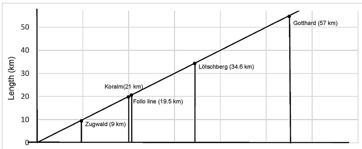
Figure 4-2: The railway tunnels from Table 4-1 which utilized TBM spoil into concrete aggregate has a minimum 10 km length, All tunnels are double barrel, except Zugwald.
