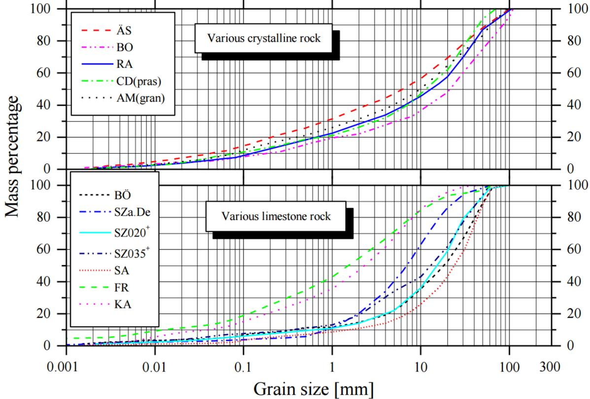
Figure 2-9: PSDs from different TBM spoils in Switzerland, sorted by crystalline or various limestone rocks [38].
