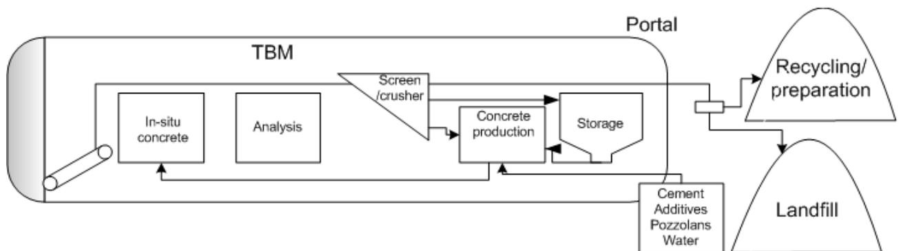
Figure 2-38: Illustrating the main procedures in the strategic plan for an automation of spoil processing [53].
