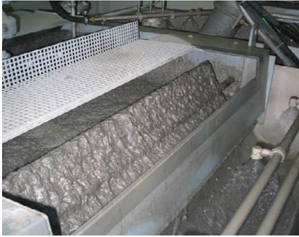
Figure 2-17: Large scale flotation was applied at the AlpTransit projects, removing the mica content in the TBM spoil fractions 63/125  $\mu\text{m}$  and 125/250  $\mu\text{m}$ [53].
