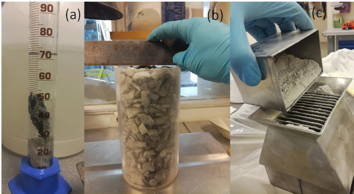
Figure 3-5: (a) Density measurement of cuttings by submerging in water. (b) Packing grade measurement. (c) Splitting of filler in preparation for the SediGraph.
