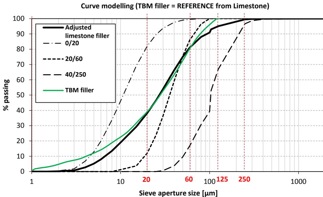
Figure 3-6: Curve modelling of limestone filler to mimic the TBM fillers. The curve “Adjusted” is a combination of 0/20, 20/60 and 40/250 µm in the ratio 47, 38, 15% respectively.
