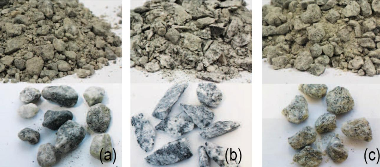
Figure 1-3: Three different 0/8 fractions from Norway. (a) The most wanted: glaciﬂuvial originated sand, (b) low quality crushed aggregates. (c) Crushed aggregates processed through a VSI, producing a product in close resemblance to the glaciﬂuvial sand
