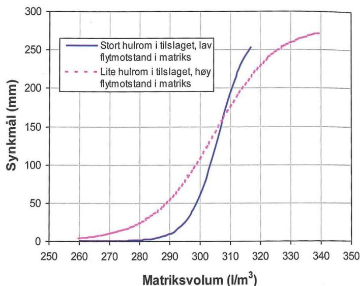
Figure 2-26: The correlation between slump value and matrix volume. Until slump values of 150 mm the most efficient slump is achieved with the so-called particle dominated mix. Slump values above 150 mm will be ruled by the matrix as it's volume is large enough to increase the spacing between aggregates [77].
