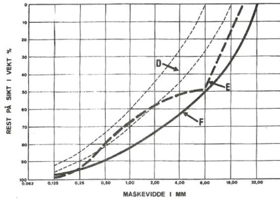
Figure 2-23: Suited PSD for different types of concrete, 0-8 mm fraction [72].
