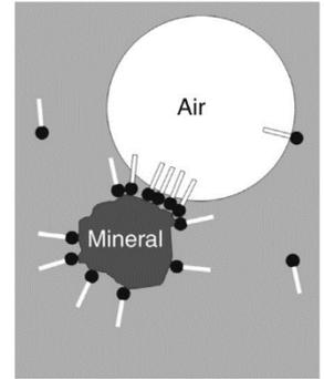
Figure2-19:Illustrating how an air bubble ascends to the surface and attaches to the hydrophobic mineral along the way (e.g. mica)[62].
