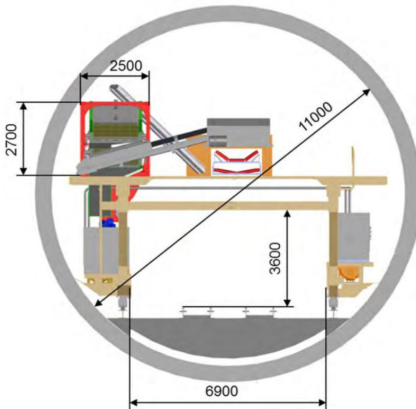
Figure 8-2: Cross-sectional view of screening unit placed inside the tunnel connected to the main conveyor belt.
