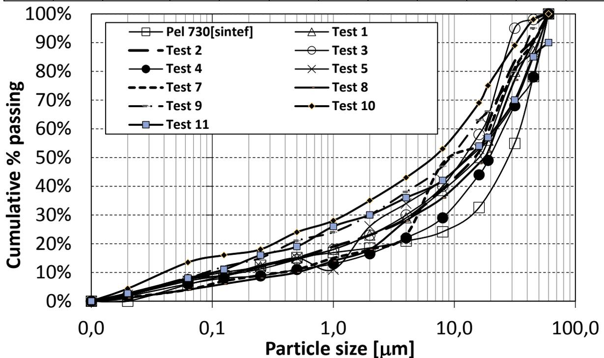
O.PSDs from Fløyfjellet TBM 1988 (source data)
