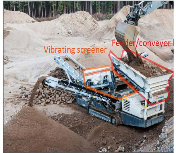
Figure 2-12: Left: Basic concept of screening through stratification and separating the feed into three fractions with a rapid separation of fines. Right, Showing Metso Scalping vibrating screener separating material into 3 different fractions [58].
