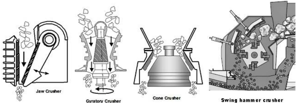
Figure 2-11: Illustration of crusher types which potentially be used in processing TBM spoil [34].
