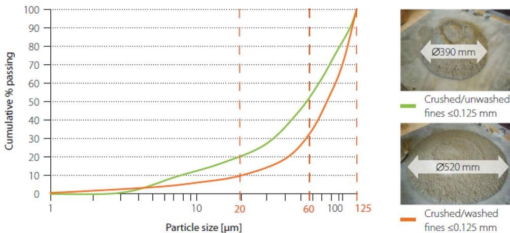
Figure 2-28: Two similar concrete recipes with  $w/c=0.5$ . Green line is unwashed filler and orange is washed filler. The differences in PSD in the filler fraction is seen to have significant impact on slump value in the fresh state. [37]
