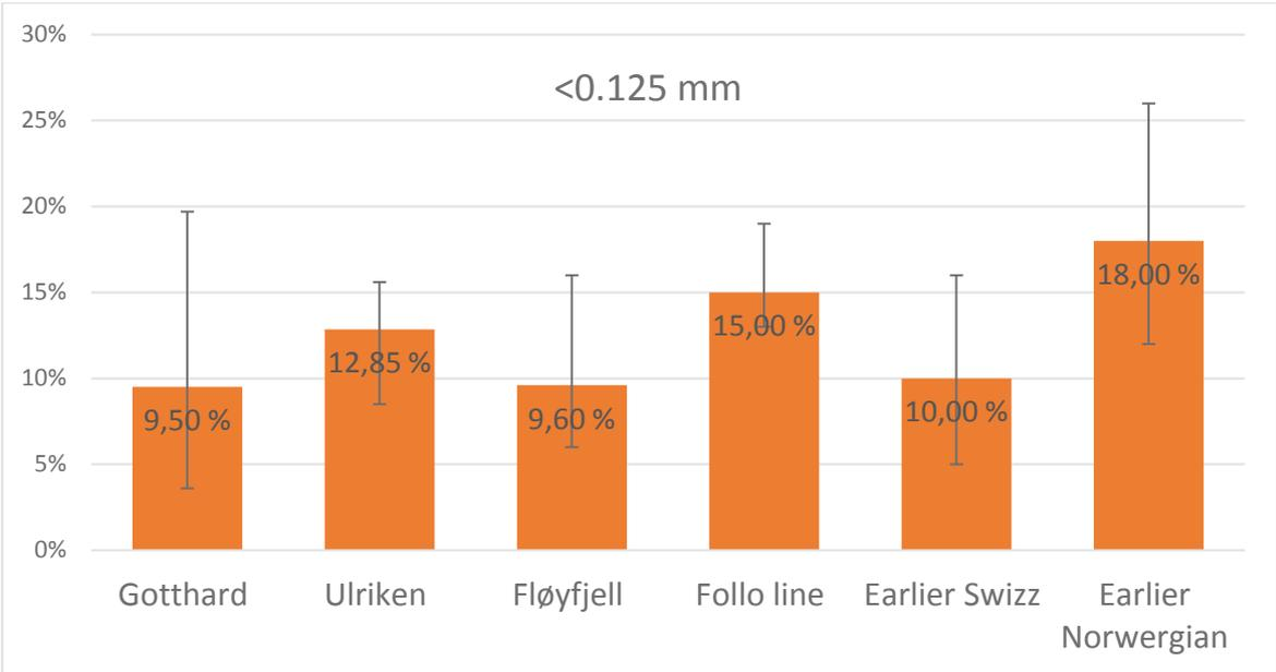
Figure 4-3: PSDs from various TBM projects and their average content of what is below the 0.125 mm sieve. The average is 11.8%.
