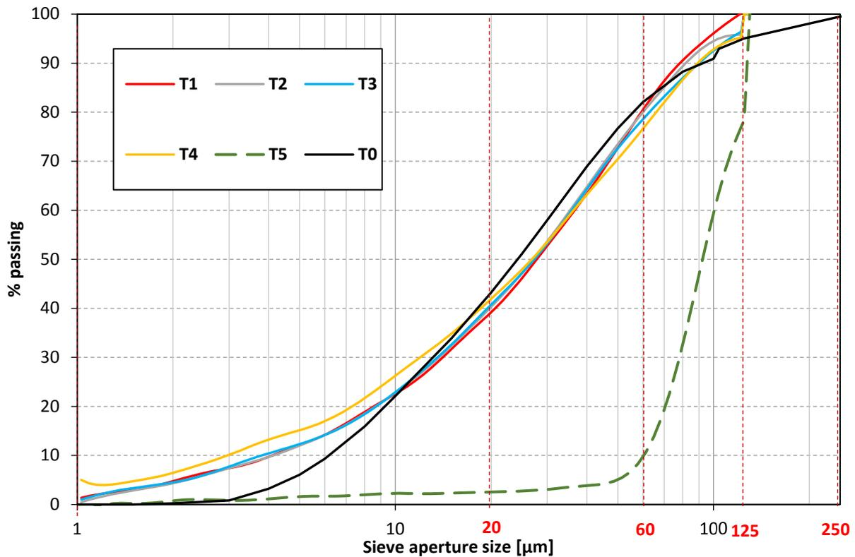
Figure 4-9: PSD of the TBM fillers from Ulriken and Follo line. The raw unprocessed TBM spoil show minor differences. It was not possible to create an identical PSD to the TBM spoil
