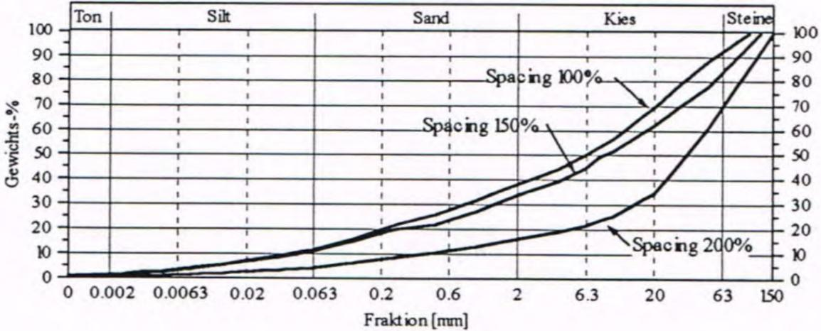
Figure 2-8: Increasing spacing between disc cutters results in a coarser PSD [53].
