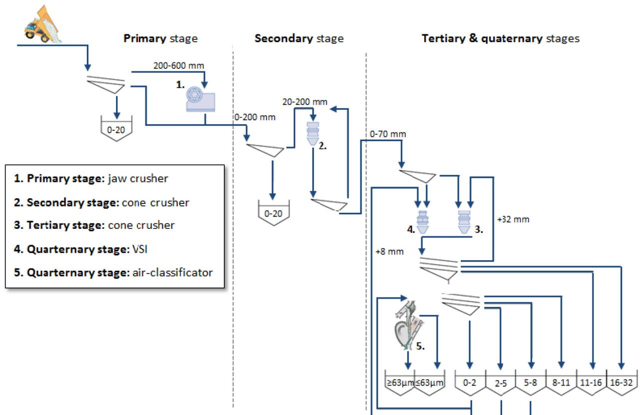
Figure 2-10: Processing of crushed sand, the quarternary stage is illustrated with a dry process , though wet processing is also possible [13].
