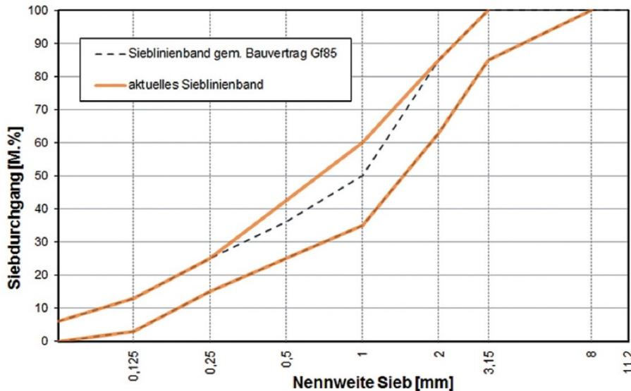
Figure 2-44: Boundary lines for the 0/8 mm fraction. The boundaries allow for high amounts below 0.125 mm [98].
