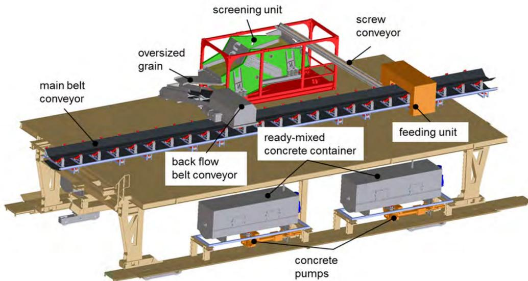
Figure 8-1: Opposite view of, now showing ready-mix concrete containers and pumps.
