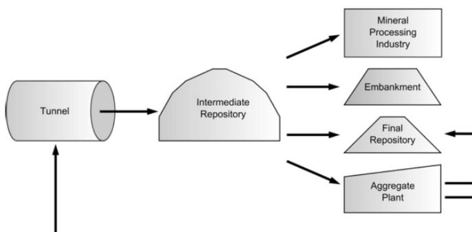
Figure 2-40:Left: general flow chart for an Swiss made approach of excavated material called TEMH( Tunnelling excavation material handling) 2012 [23, 33].
