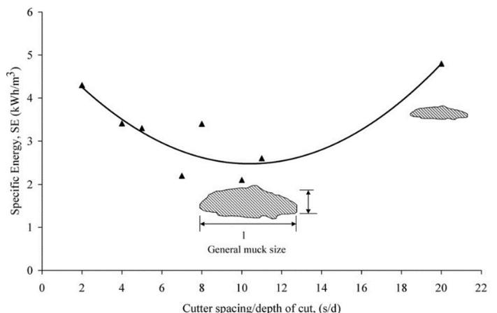
Figure 2-7: Left From the muck buckets the spoil is carried on to the conveyer system by closed gutters. Wetting of the conveyer belt is also used to lower the dust development inside the tunnel[53]. Right: Relationship between specific energy of the TBM cutter head versus spacing/cutter depth ratio. Largest PSD was obtained with a cutter spacing of 75 mm[27].
