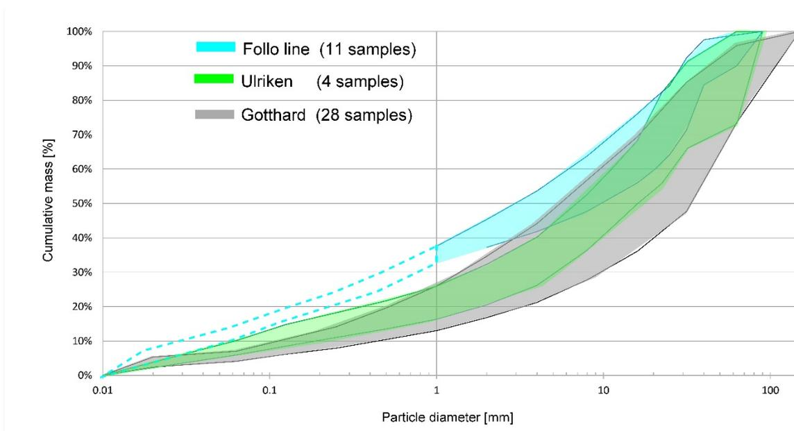
Figure 4-1: Follo line, Ulriken and Gotthard compared on its normalized PSDs, the extremes are removed. Follo line: Predicted content below 1 mm is marked with dotted lines due to missing data.
