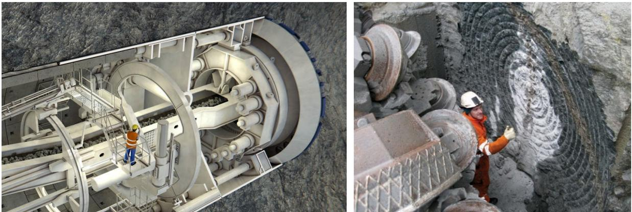
Figure 2-1 Left: Illustration of a double shield TBM[42]. Right: An engineer is inspecting the tunnel at a project at Faroe Island in 2010. The spacing and penetration is visible in the rock face [43].
