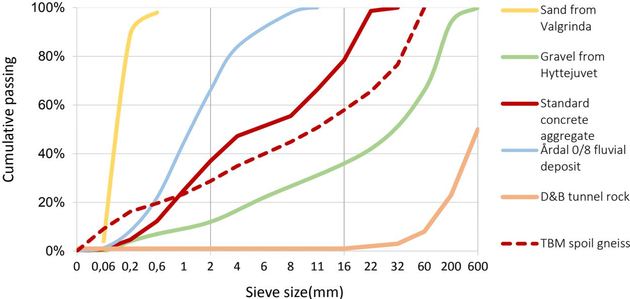
Figure 1-2: The PSDs illustrates the TBM spoils close resemblance to concrete aggregates in comparison to other granular sources.
