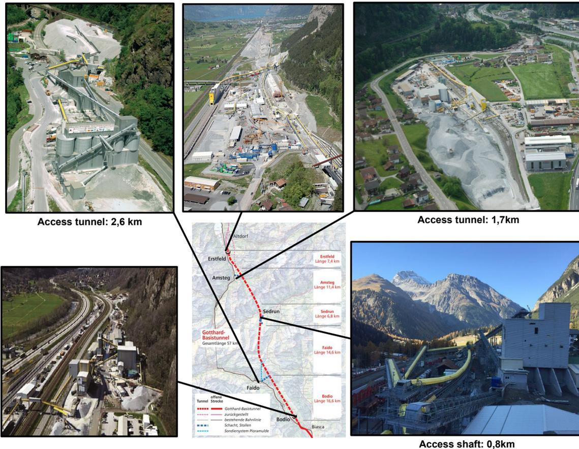
Figure 2-35: The Gotthard tunnel illustrating the three intermediate access tunnels and two portals. Erstfeld, Amsteg, Sedrun, Faido and Bodio. Actual aggregate processing happened at Amsteg and Bodio [55].
