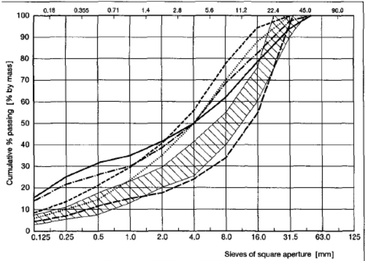
Fig. 1 – Particle size distribution of the 5 TBM materials (shaded area within SIA standard 162, art. 5, 14, 24; Fuller).
