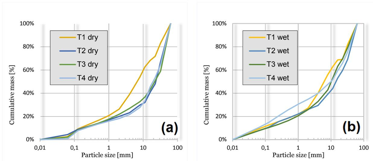
Figure 4-7: 1 kg PSD measurements of the TBM spoil, wet and dry sieved technique applied.
