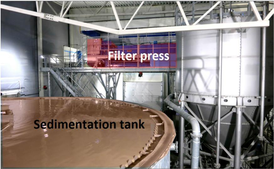
Figure 2-16: At the Follo line project (figure) and AlpTransit projects the cleansing of sludge from the wet processing of TBM spoil was done by a clarifier (sedimentation tank) and a VPA (filter press) creating filter cakes of mud for the landfill. The partially cleansed water can be used back in the wet processing.
