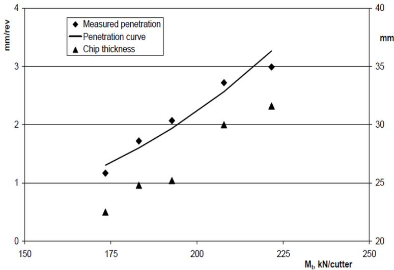
Figure 2-6: Increasing chip thickness with increasing penetration in a mica gneiss [49].
