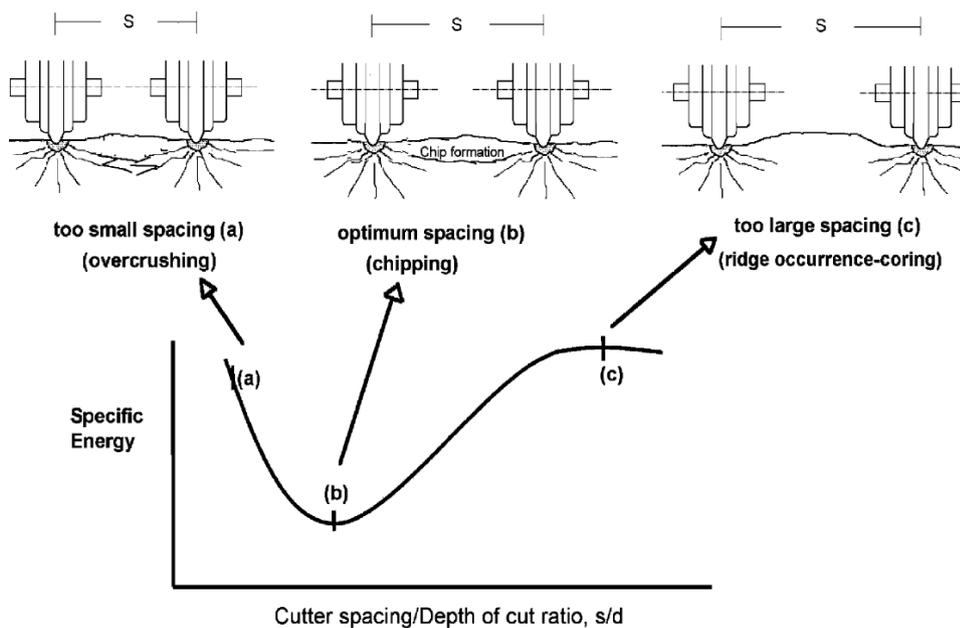
Figure 2-5. Right: The optimum cutting efficiency is closely related to the cutter spacing/penetration ratio and specific energy [27].
