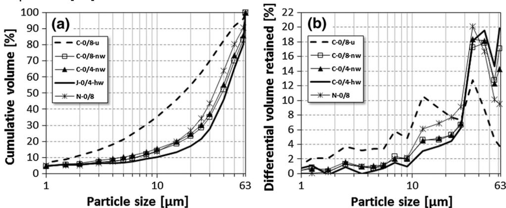
Figure 2-30: (a) PSD measurements with X-ray sedimentation method. (b) presented by difference in volume [83] C-0/8-u = crushed unwashed
