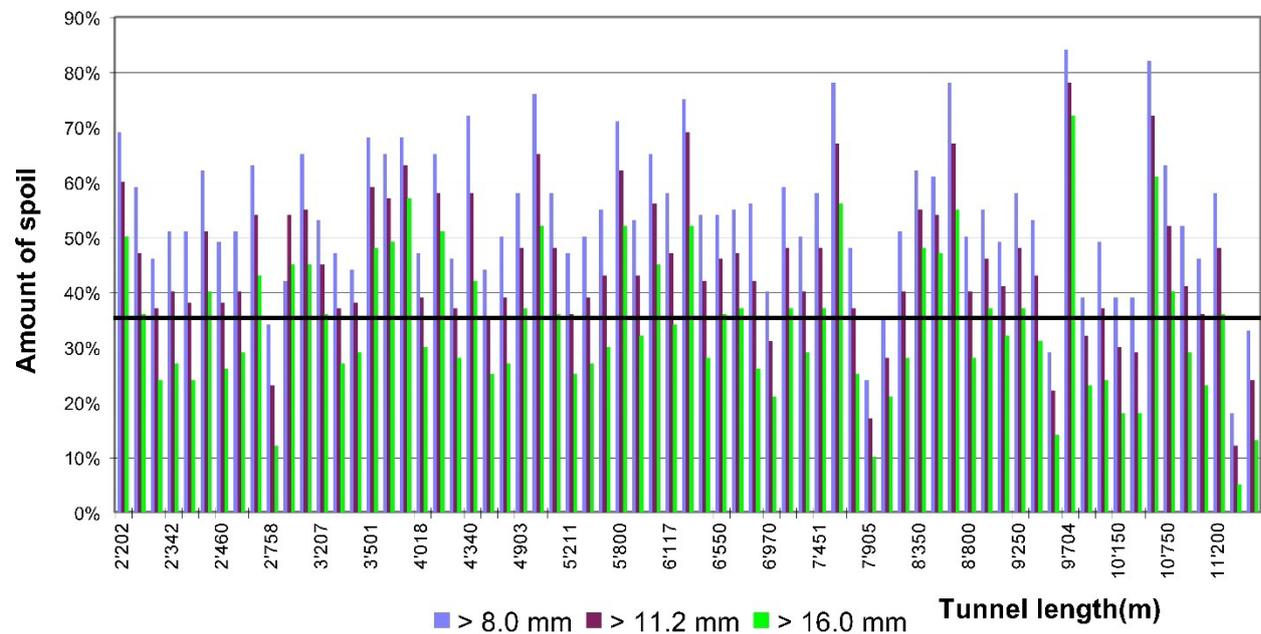
Figure 2-43: The TBM spoil excavated over a period of 9,5 km in the Zugwald tunnel. The black horizontal line are the average of >16 mm , which was 34 % [36].
