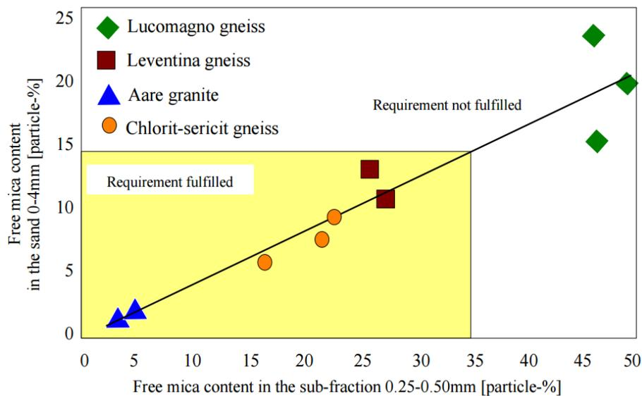
Figure 2-20: Correlation between free mica content in 0/4 mm and 0.25/0.5 mm fraction. Yellow zone represents a sand which have fulfilled B30/40 concrete [33].
