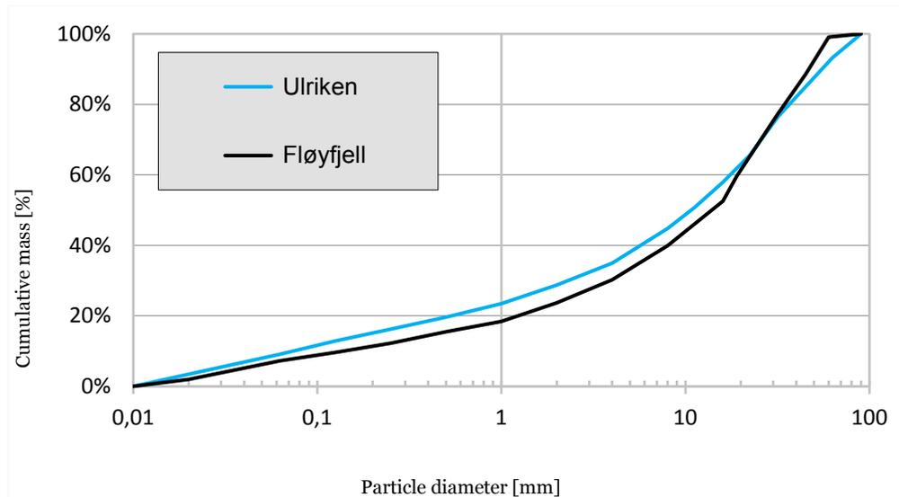
Figure 4-4: Comparing the average of PSDs from TBM projects Ulriken and Fløyfjell.
