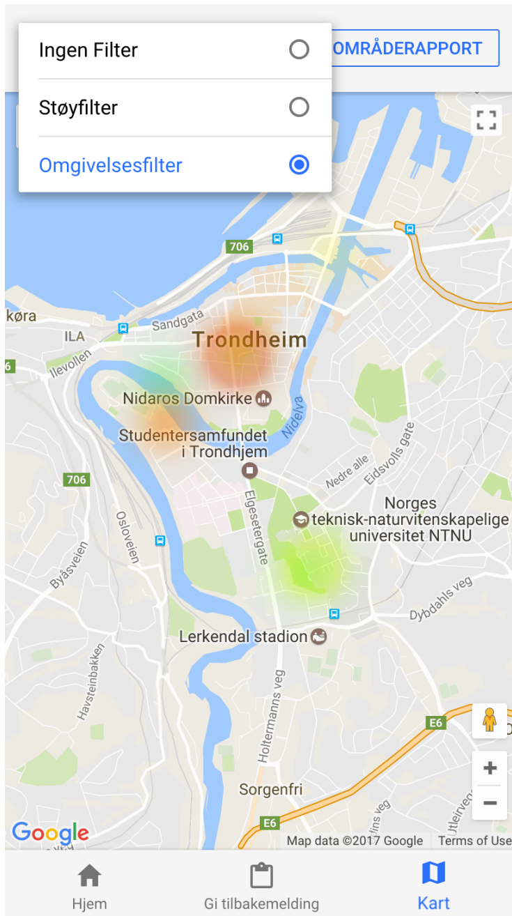
Figure 7.10: Screenshot of the heat-map with noise level selected as the filter.
