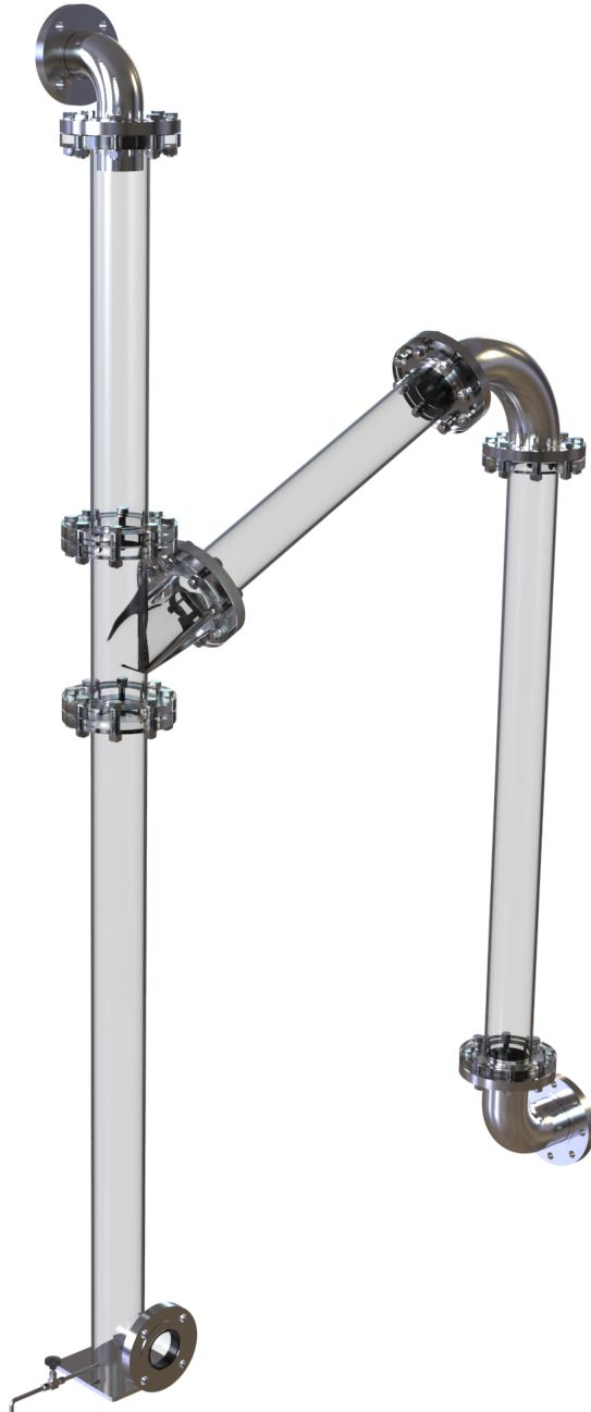
Figure 3.27: The final GLCC constructed in transparent PVC and 316L.
