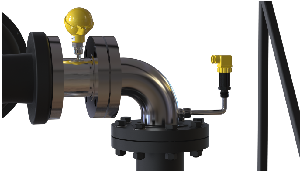
Figure 4.12: Pressure transmitter 3-PT-102 and the temperature transmitter 3-TT-202 located at the gas outlet of the GLCC.
