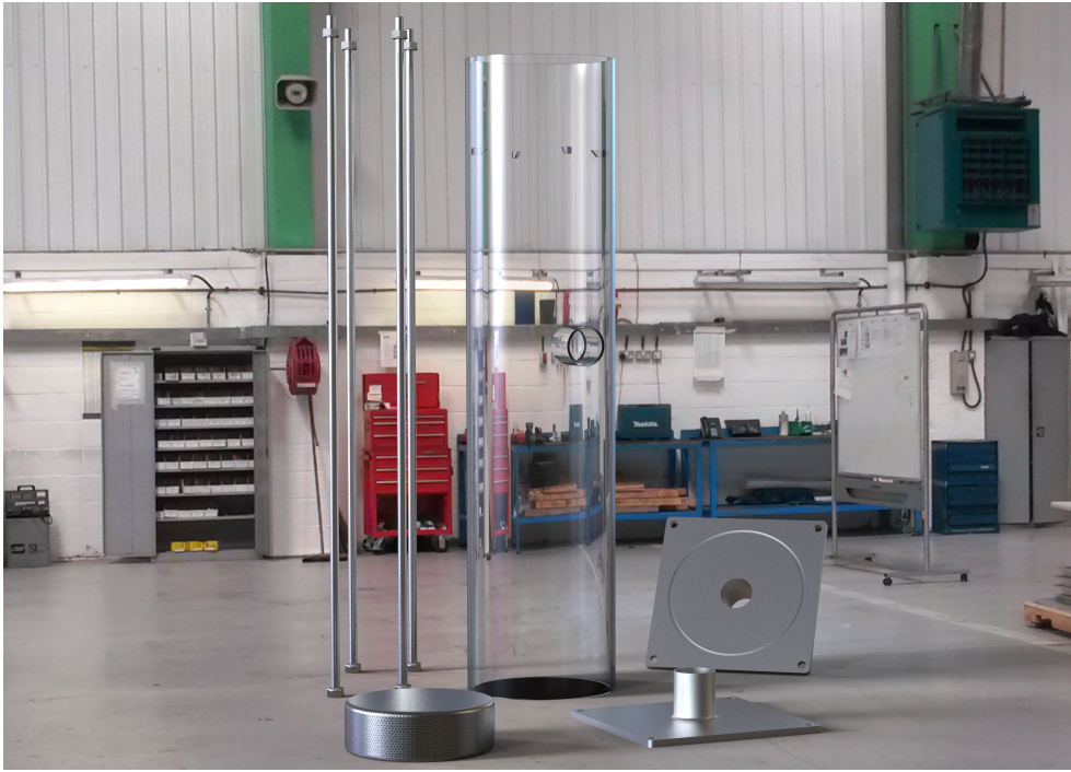
Figure 6.2: Illustration of scrubber sections after manufacturing. The background is retrieved from Keyshot 6 software.
