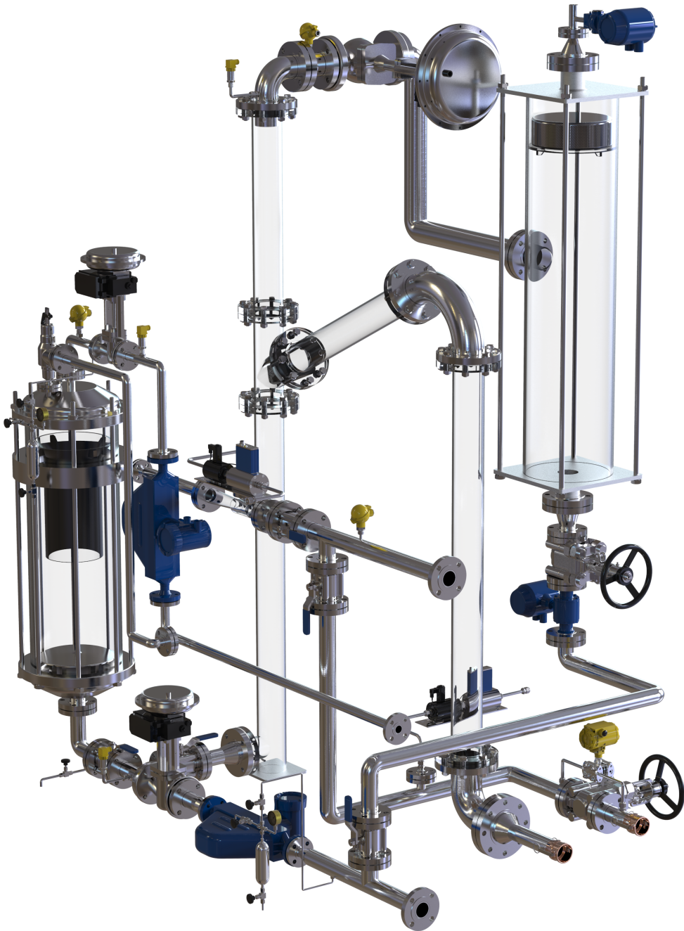
Figure 4.4: Phase 2 process equipment illustrated without steel frame or nitrogen gas reservoir.
