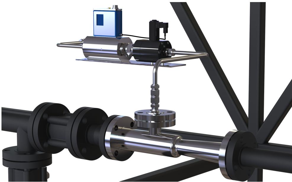
Figure 4.10: CFU nitrogen gas injection by mixer and Ex-flow unit. The homogeneous mixed phase flows to the right.
