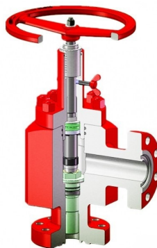
Figure 2.17: Illustration of Choke Valve [12]
