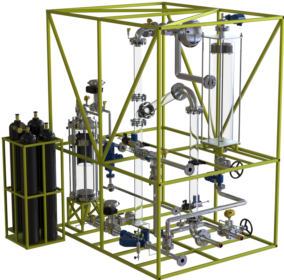
Figure 4.3: Final design of Phase 2 including steel frame, process equipment and gas reservoir.
