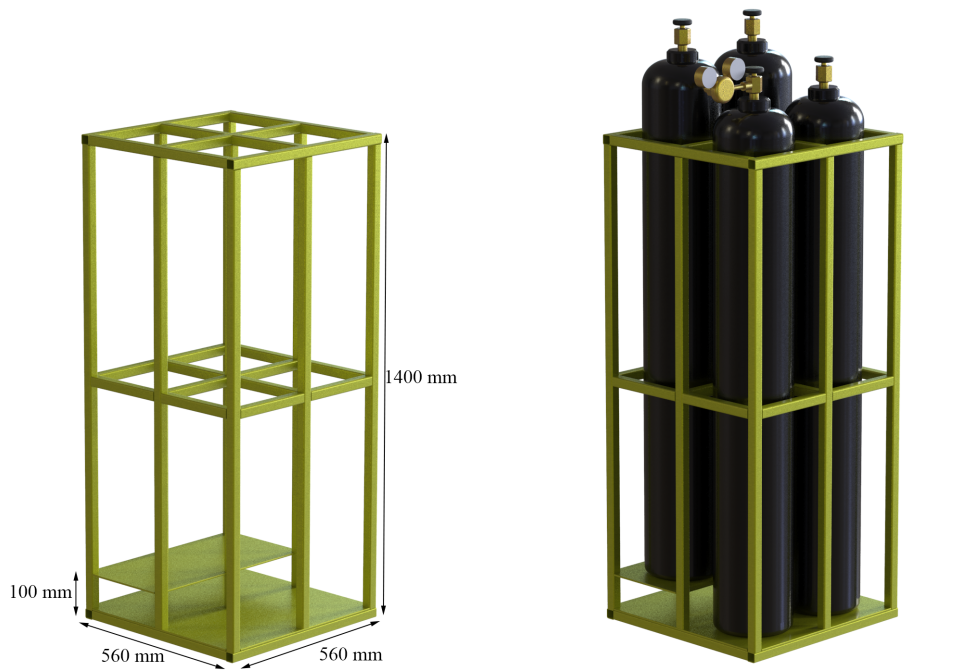
(a) Gas reservoir holding cage. The cage can contain four bottles of 50 liter nitrogen gas pressurize at 200 bar.
