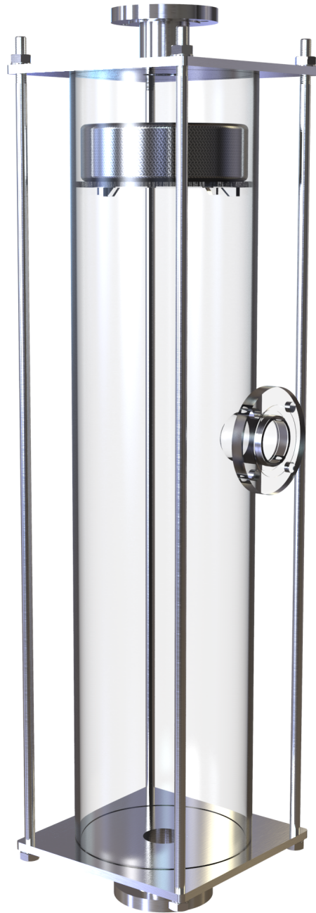
Figure 3.36: The final Scrubber constructed in transparent PVC, 316L and aluminum.
