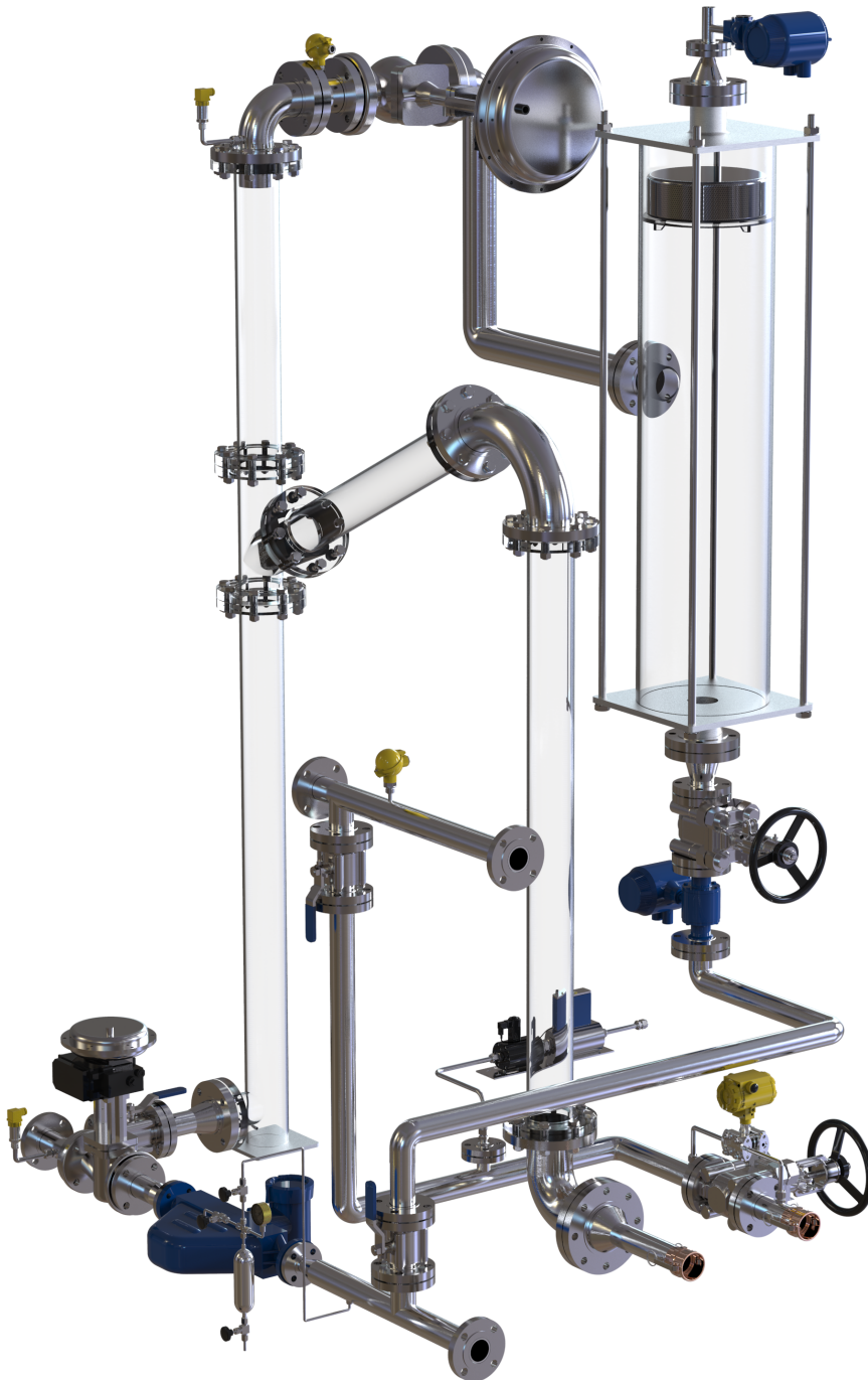
Figure 4.13: GLCC process equipment.
