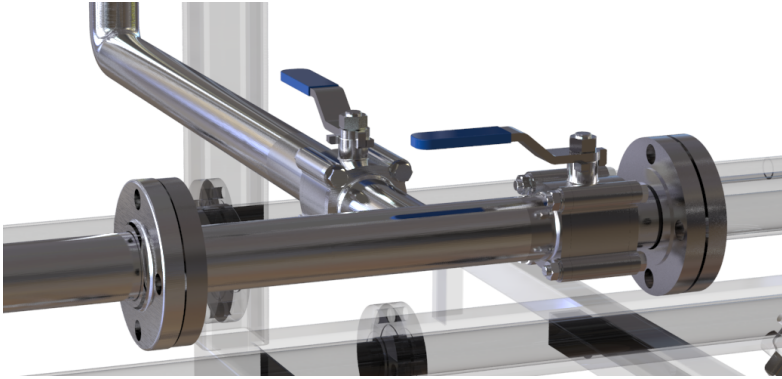
Figure 4.24: Process feed diverting between Phase 1 and Phase 2. Phase 1 pipes are transparent for illustrative purposes.
