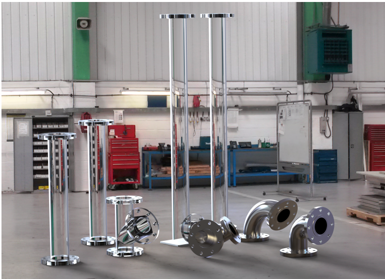
Figure 6.1: Illustration of GLCC sections after manufacturing and partial assembly. The background is retrieved from Keyshot 6 software.
