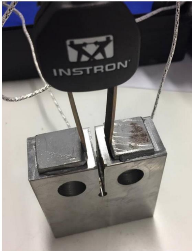
FIGURE 2 - INSTRON CRACK OPENING DISPLACEMENT GAUGE MOUNTED ON FATIGUE CRACKING SAMPLE
