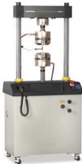
FIGURE 1- INSTRON 8801 SERVOHYDRAULIC TEST RIG USED FOR TENSILE AND FATIGUE TESTS [2]
