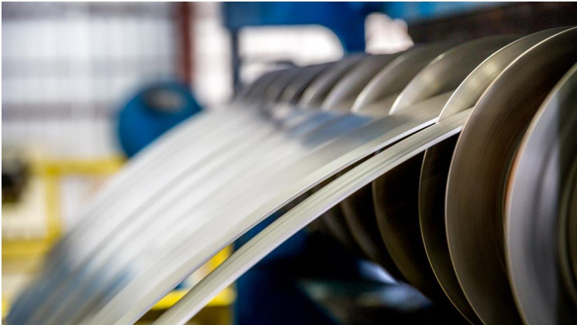
FIGURE 12 - SLITTING STEEL SHEETS FOR CT [10]
