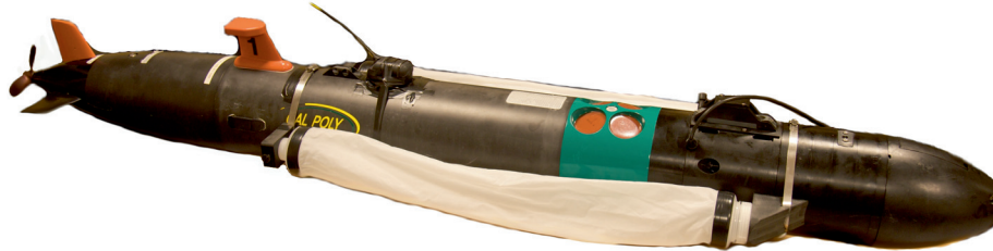
Fig 4. The REMUS-100 AUV. The green section with red circles is the ADCP (upward- and downward-looking). The nose cone contains the BP, and the organisms passing through the BP detector are captured by the attached plankton nets. Photo: Geir Johnsen.
