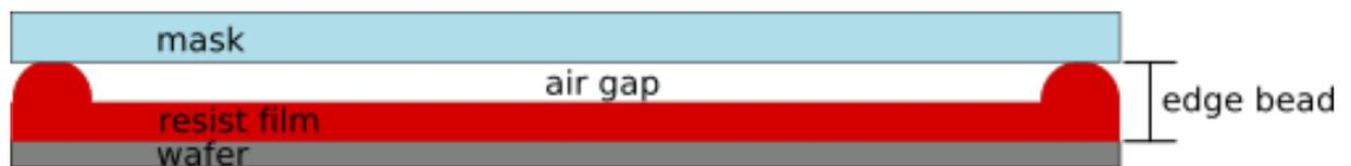
**Figure 5.3-6. The effect of edge bead on hard contact exposure.** The edge bead will be brought into contact with the mask, leaving an air gap between the mask and the substrate. There is also significant risk of mask contamination.
