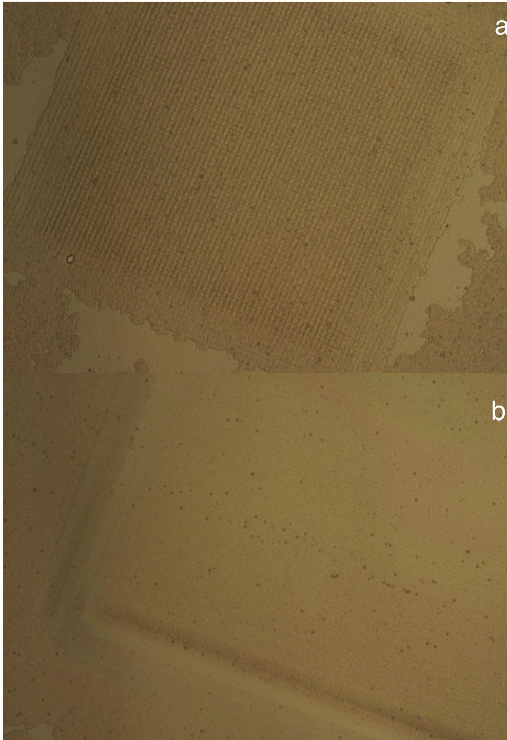
**Figure 5.3-1. Silicone wafers with SU-8 2003.5 covered in residue formed after development in MrDEV-600.** The patterns shown are (a)  $10 \times 10 \mu\text{m}$  squares with a  $10 \mu\text{m}$  separation distance and (b)  $8 \mu\text{m}$  stripes with an  $8 \mu\text{m}$  separation distance. The images were obtained using a Nikon Eclipse LV150 microscope.
