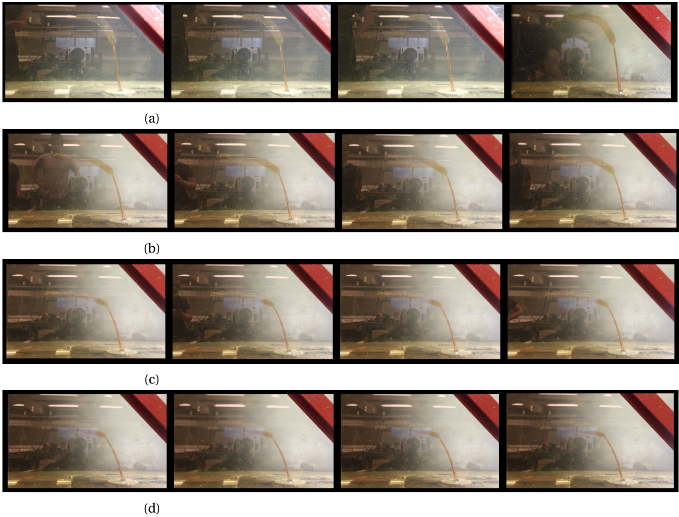
Figure A.3: Motions from the model test of the surrogate 90A (a) 0.05\text{ m/s} , (b) 0.14\text{ m/s} , (c) 0.17\text{ m/s} , and (d) 0.21\text{ m/s} .
