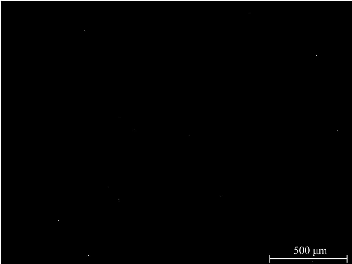
Figure 4.34: Dark field optical microscopy image of substrate A after a Br:methanol etch taken near the centre of the substrate.
