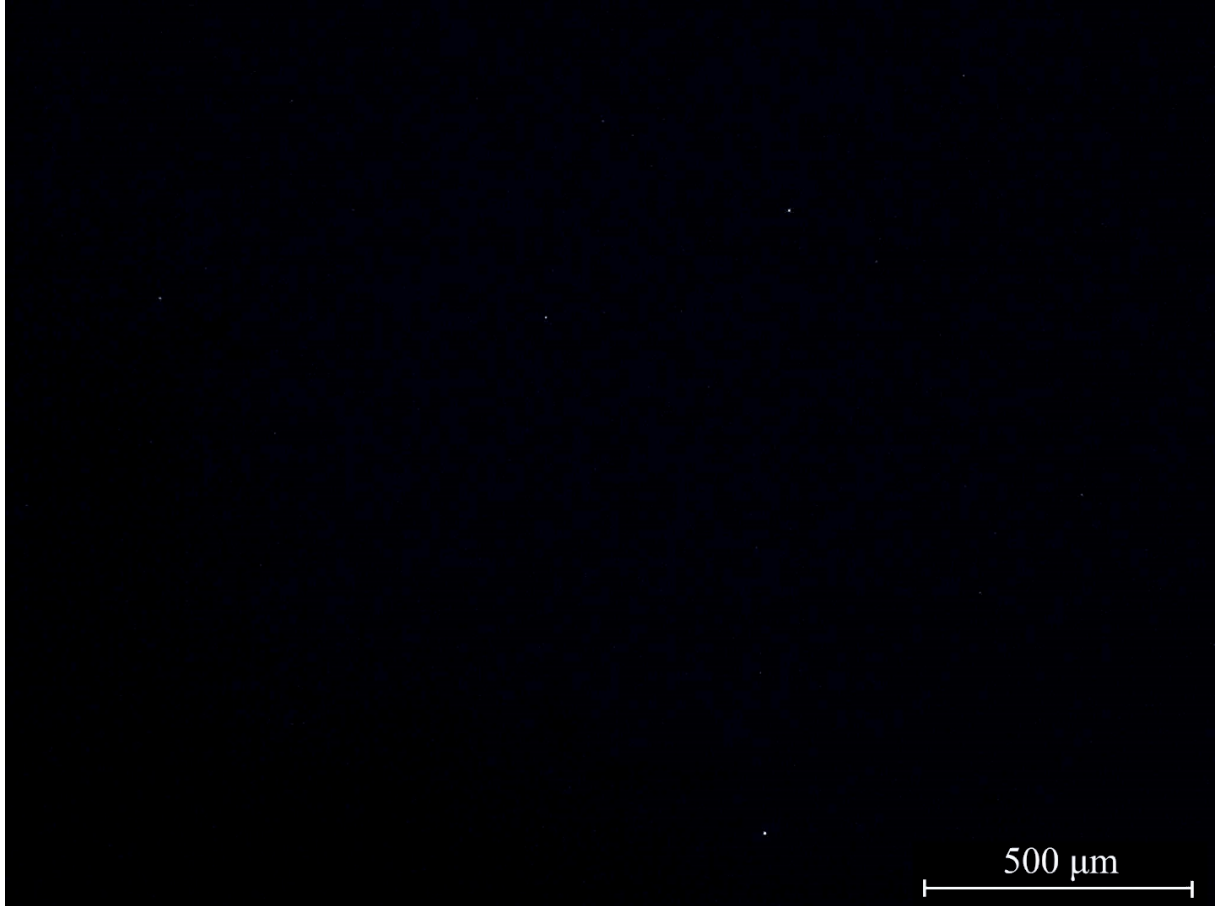
Figure 4.1: Dark field image of substrate A captured through the optical microscope Leica DM RXA2 at the centre of the substrate surface.
