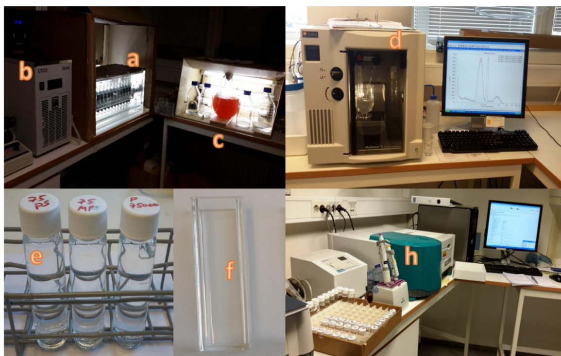
Image 1. Some of the instruments used during experimentation. The experimental system is made up of a), the plankton wheel, b) heating/cooling bath to maintain the temperature of the plankton wheel's water bath constant, c) batch culture, d) Beckman coulter counter. e) the 40mL culture vials, f) square spectrophotometer cuvette and h) the Cary Eclipse fluorescence spectrophotometer.
