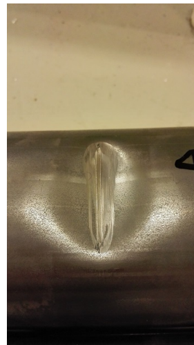
(b) Dent with Gouge
