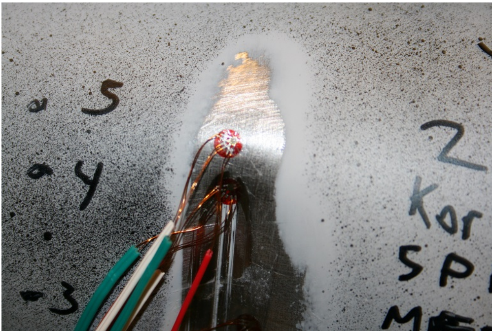
Figure 5.32: Misplacement of Gage 5 in Test 5
