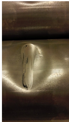
(a) Dent without Gouge
