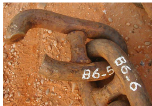
Figure 2.17: Link failure on a deep water buoy due to OPB (Rampi, Dewi, Francois, Gerthoffert and Vargas, 2016)
