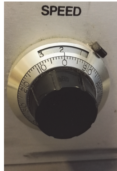
Figure 1-7 Engine speed knob, dialed to 20 rps
