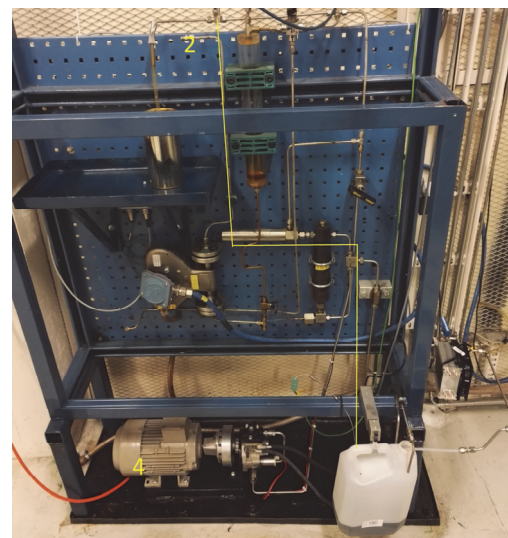
Figure 8-11 Location of improvement nr.2 and 4. Yellow line is proposed route for fuel return.
