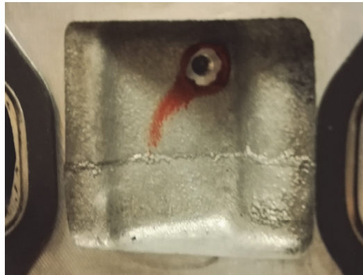
Figure 8-1 Sealed hole behind exhaust manifold
