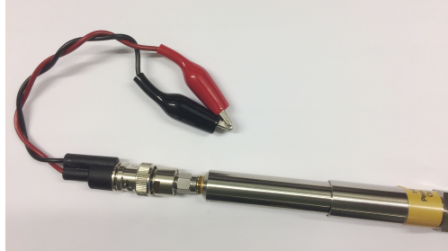
Figure 4.10: Short circuit test of probe.
