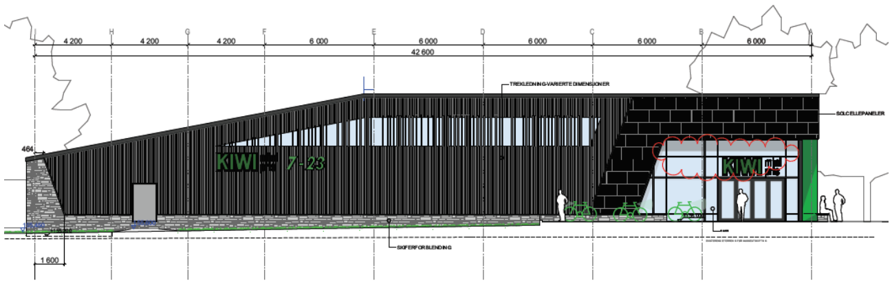
Figure 51: KIWI Dalgård - Planned PV area on the northwestern facade, marked by black facade panels
