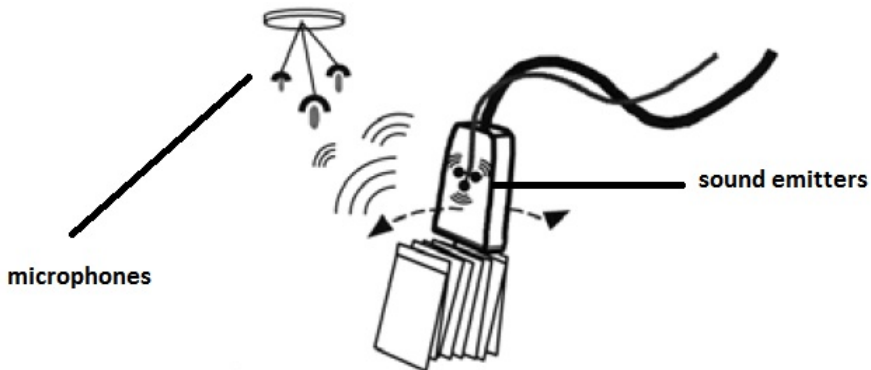
Figure 7: Acoustic 3D scanning
