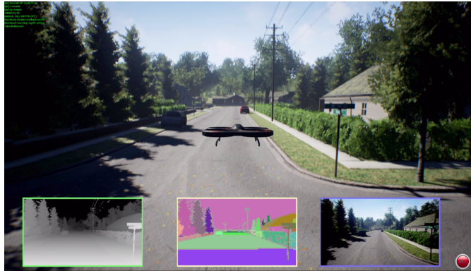
(a) Flying a multirotor in Microsoft AirSim. The three boxes at the bottom are depth camera, depth segmentation, and First Person View (FPV)
