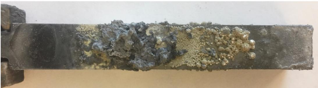
**Figure 6.1:** Composite sample 3018g after completed wetting test.
