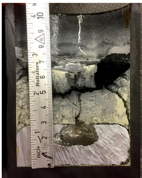
**Figure 4.5:** Cross-section of crucible with solidified electrolyte and metal after completed wetting test.
