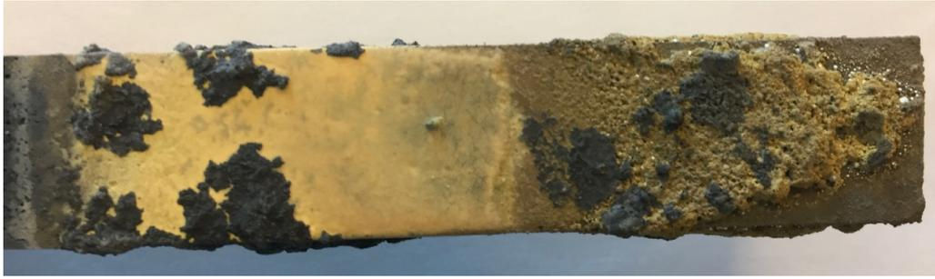
**Figure 6.7:** Composite sample 5020g after completed wetting test.
