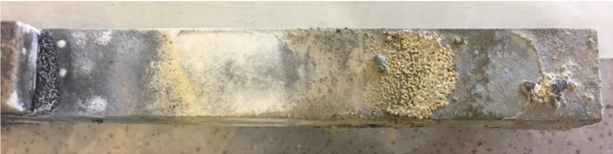
**Figure 6.3:** Composite sample 3112g after completed wetting test.
