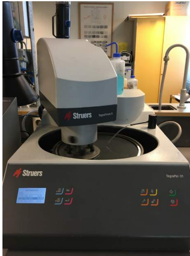
Figure 36: Struers TegraPol-31 for automatic grinding and polishing of the samples
