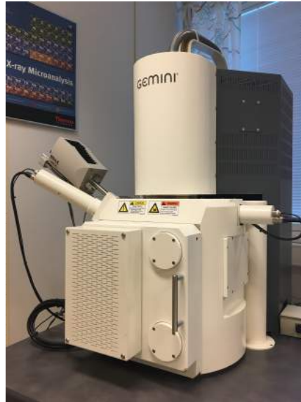
Figure 38: External view of the SEM used in this work
