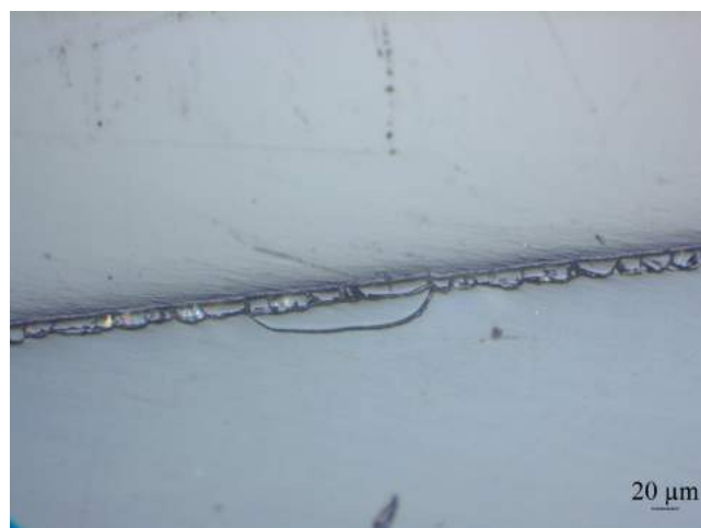
Figure 131: Cristobalite layer observed on A_n after HT1 of 10 h : Thin occurrence, homogeneous
