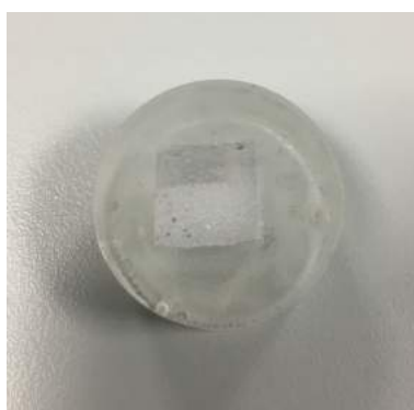
Figure 35: Epoxy embedded quartz sample, cross section oriented
