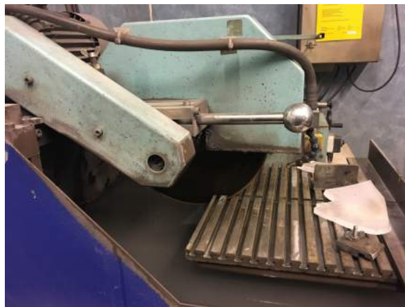
Figure 24: Rough diamond saw: Side view with the rough blade and the mobile sample holder
