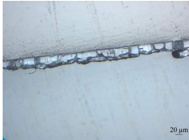
Figure 143: Cristobalite layer observed on A_{nc} Piece 3 (above the melt) after HT2 of 10 h : Thin occurrence, homogeneous
