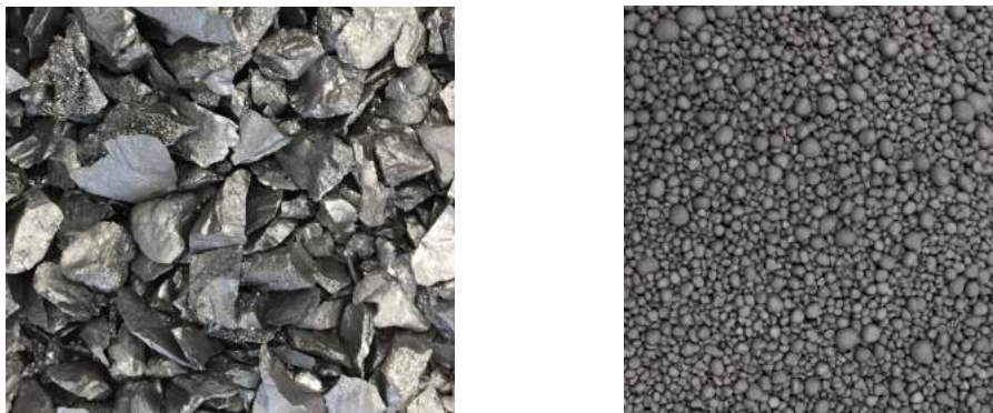
Figure 4: Pictures of Si chunks from the Siemens process (left) and Si granules from the FBR process (right), both from NTNU resources
