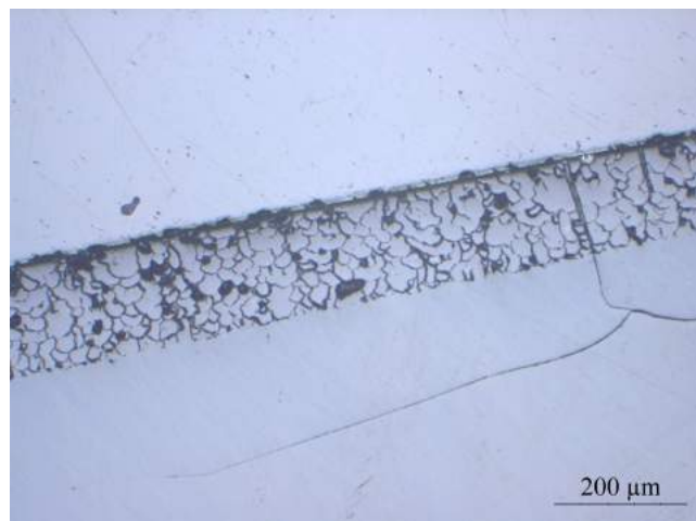
Figure 142: Cristobalite layer observed on Std_{nc} after HT1 of 24 h : Large occurrence, very homogeneous
