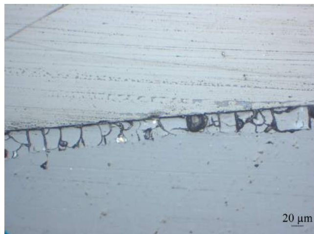
Figure 144: Cristobalite layer observed on A_{nc} Piece 2 (in the melt) after HT2 of 10 h : Larger occurrence, homogeneous
