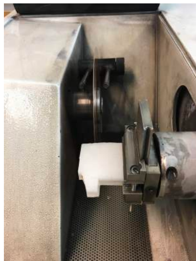
Figure 25: Precise diamond saw: Cutting chamber with mobile sample holder and fine blade
