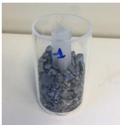
Figure 29: Sample set-up for HT1: 4 cm long quartz rod in 40 g Si chunks
