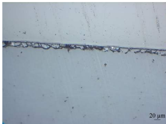
Figure 134: Cristobalite layer observed on Std_{nc} after HT1 of 10 h : Thin occurrence, homogeneous
