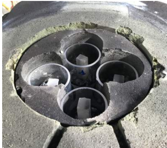
Figure 30: Furnace set-up for HT1: The 4 crucibles placed in the insulation parts
