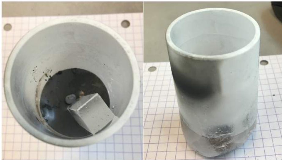
Figure 67: Resulting crucibles from HT1 of 10 h at high temperature
