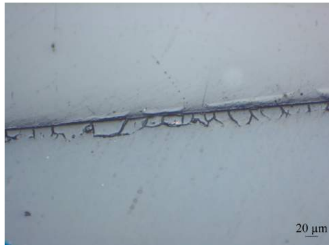
Figure 132: Cristobalite layer observed on B_n after HT1 of 10 h : Thin occurrence, homogeneous
