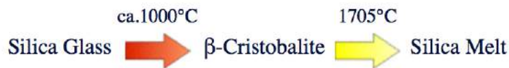
Figure 11: Successive phase transitions of high purity fused quartz crucibles made of silica glass with increasing temperature [7]
