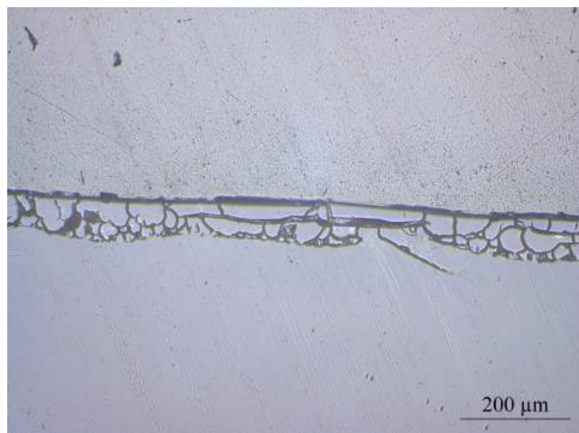
Figure 129: Cristobalite layer observed on B_n spray coated after HT1 of 90 min : Thicker occurrence, homogeneous
