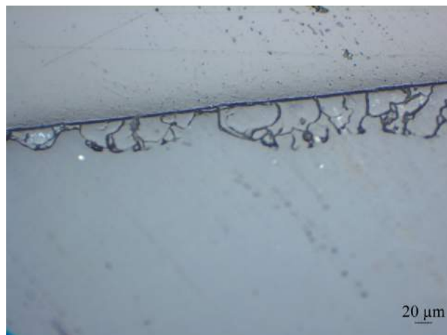
Figure 133: Cristobalite layer observed on B_{nc} after HT1 of 10 h : Larger occurrence, quite homogeneous
