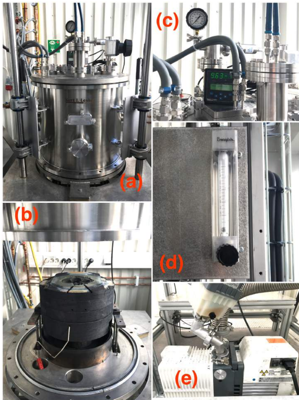
Figure 31: VGF elements: Sealed furnace (a); open furnace with graphite parts and sample holder (b); manometers (c); argon flowmeter (d); vacuum pump (e)
