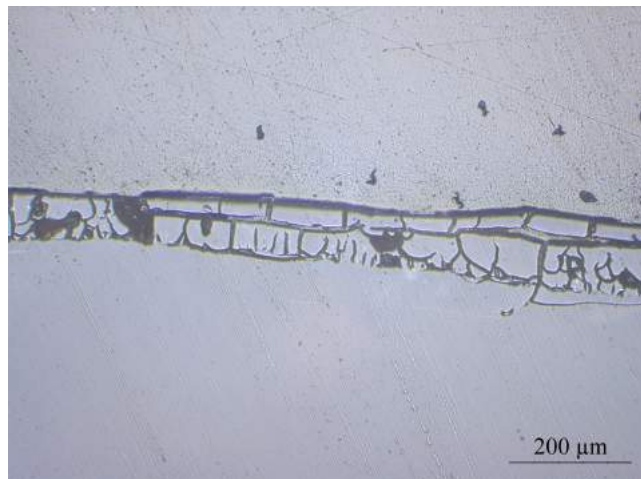
Figure 128: Cristobalite layer observed on A_n spray coated after HT1 of 90 min : Thicker occurrence, homogeneous
