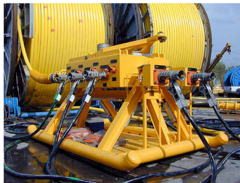
Figure 2.14: Umbilical Termination Assembly (UTA) [17].
