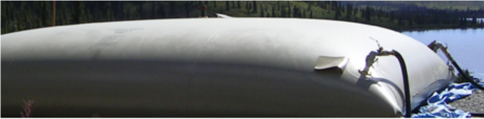
Figure 2.8: Pillow tank (Sei Industries Ltd., 2016).
