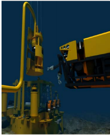
Figure 2.25: Vertical connection system (FMC Technologies, 2017c).
