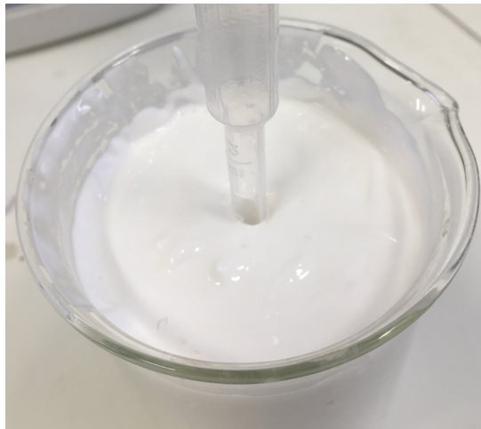
Figure 5.20: Soybean oil emulsion mixed too long, becoming very viscous
