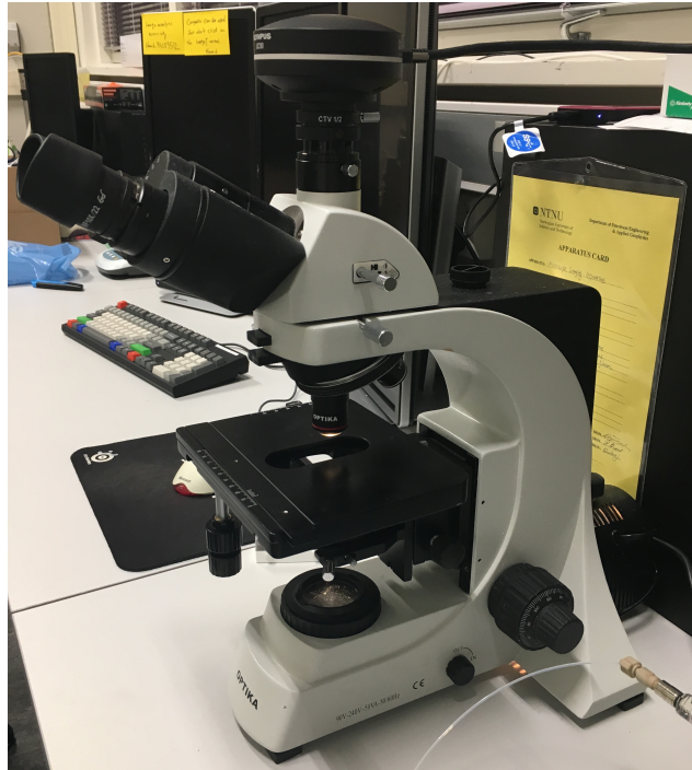
Figure 4.25: Optika microscope connected to Olympus UC90 microscope digital camera
