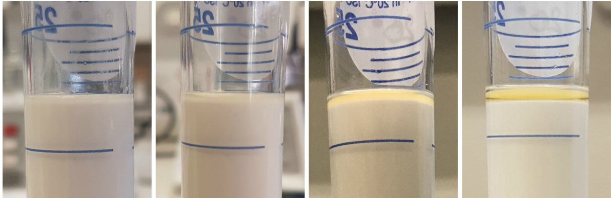
Figure H.1: Visual separation of a E30-70 emulsion in temperature 20 °C, time from left to right is 3, 4, 10 and 12 days
