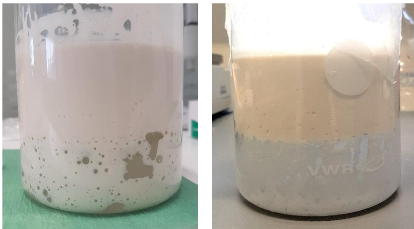
Fig. 3-3: 70/30 W/O emulsion. Straight after making (left) and 22 hours later (right)
