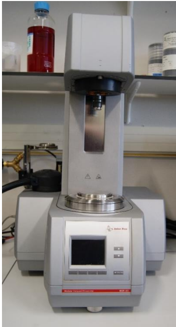
Fig. 3-7: Anton Paar Rheometer used to measure the apparent viscosity and rheology of the emulsions
