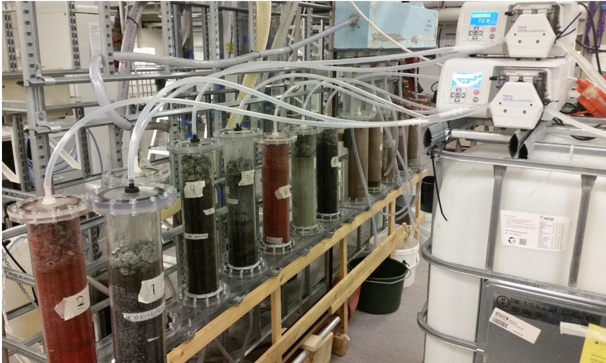
Figure 6. Experimental setup. 1 m 3 tank with synthetic stormwater down to the right. Pumps above it with tubing going from the tank to the columns lined to the left.
