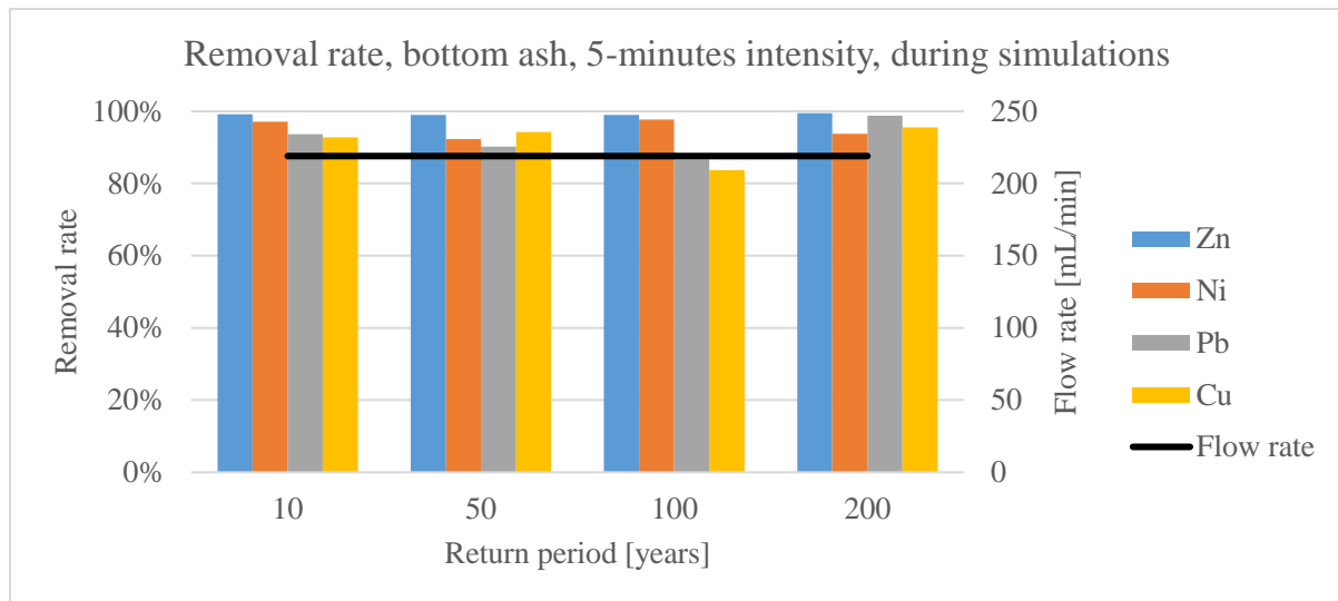
Figure 31. Removal rate of olivine during simulations of 5-minutes intensity precipitation events. Flow rate – HLR used during simulation.
