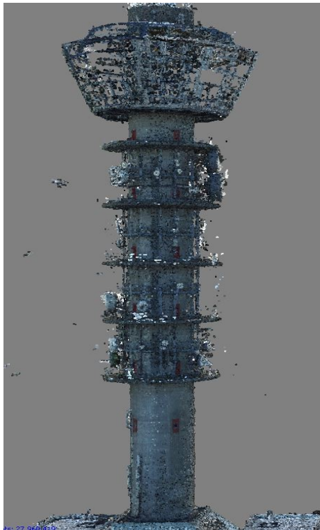
Figure 3.17 Generated Dense Point Cloud, Agisoft PhotoScan Professional
