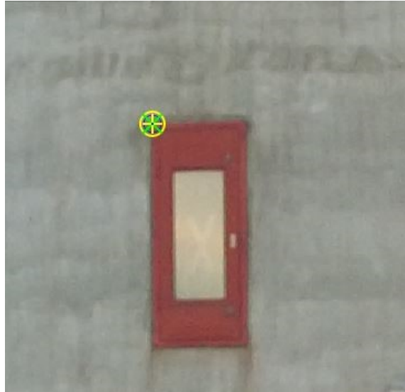
Figure 3.2 Ground Control Point marked on a photo, Pix4Dmapper Pro
