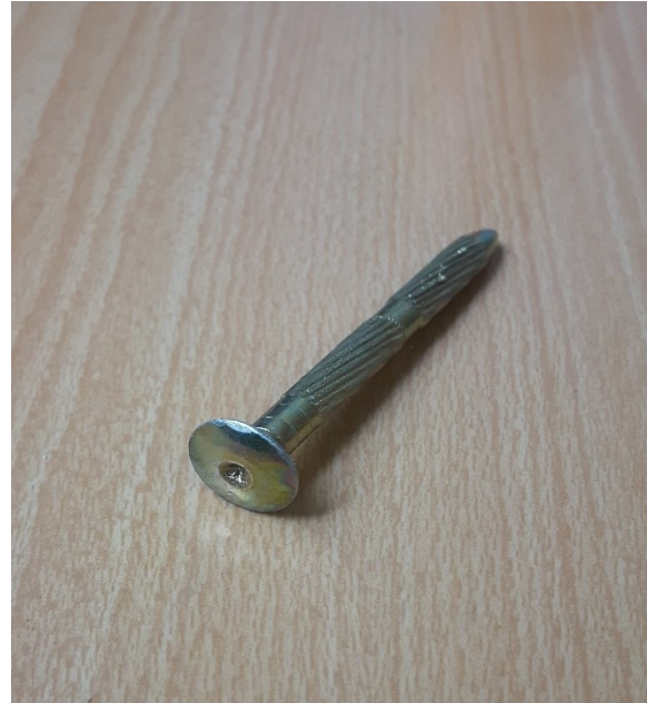
Figure 1.5 Control point nail
