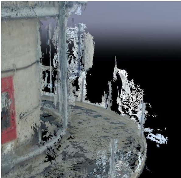
Figure 3.15 Point cloud outliers, Minimum 4 Matches
