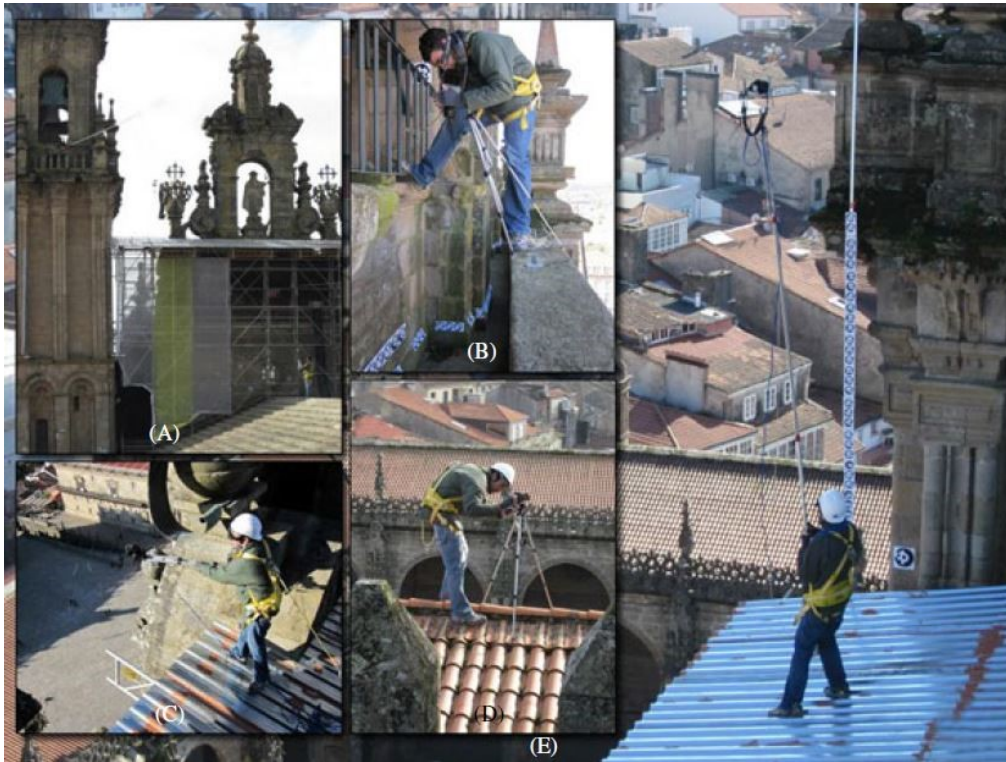
Figure 2.19 Taking photos on the roof. A shows scaffolding. B, C, D and E show capturing photos with use of tripod and telescopic lift (Martinez, Ortiz, Gil, Rego,2013)
