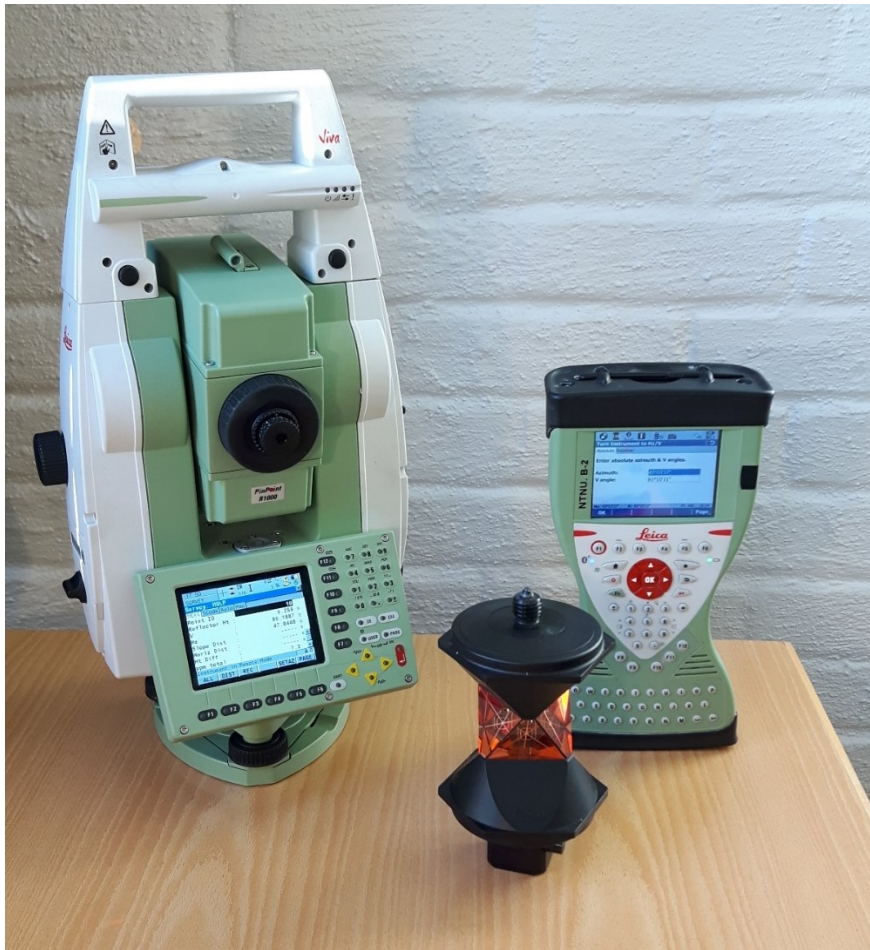
Figure 2.2 Used Total Station (Leica TCRP1201), Controller (Leica CS15) and 360 prism (Leica GRZ4).
