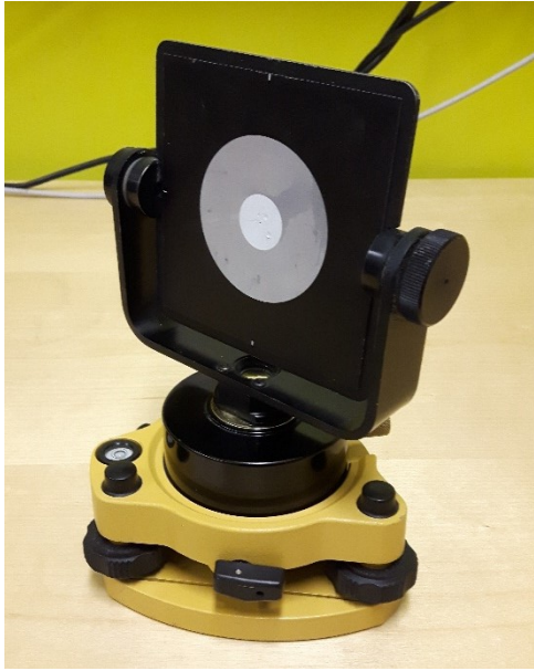
Figure 3.6 Topcon GLS-1000 Target on a tribrach
