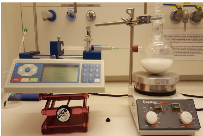
Figure 4: TEOS solution added dropwise to the round bottom flask with the use of a syringe pump, a 10 ml syringe and a horizontal opening in the flask.
