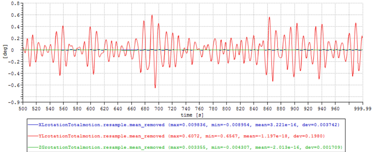
Figure 5.9: Rotational displacement of the vessel - Test 4
