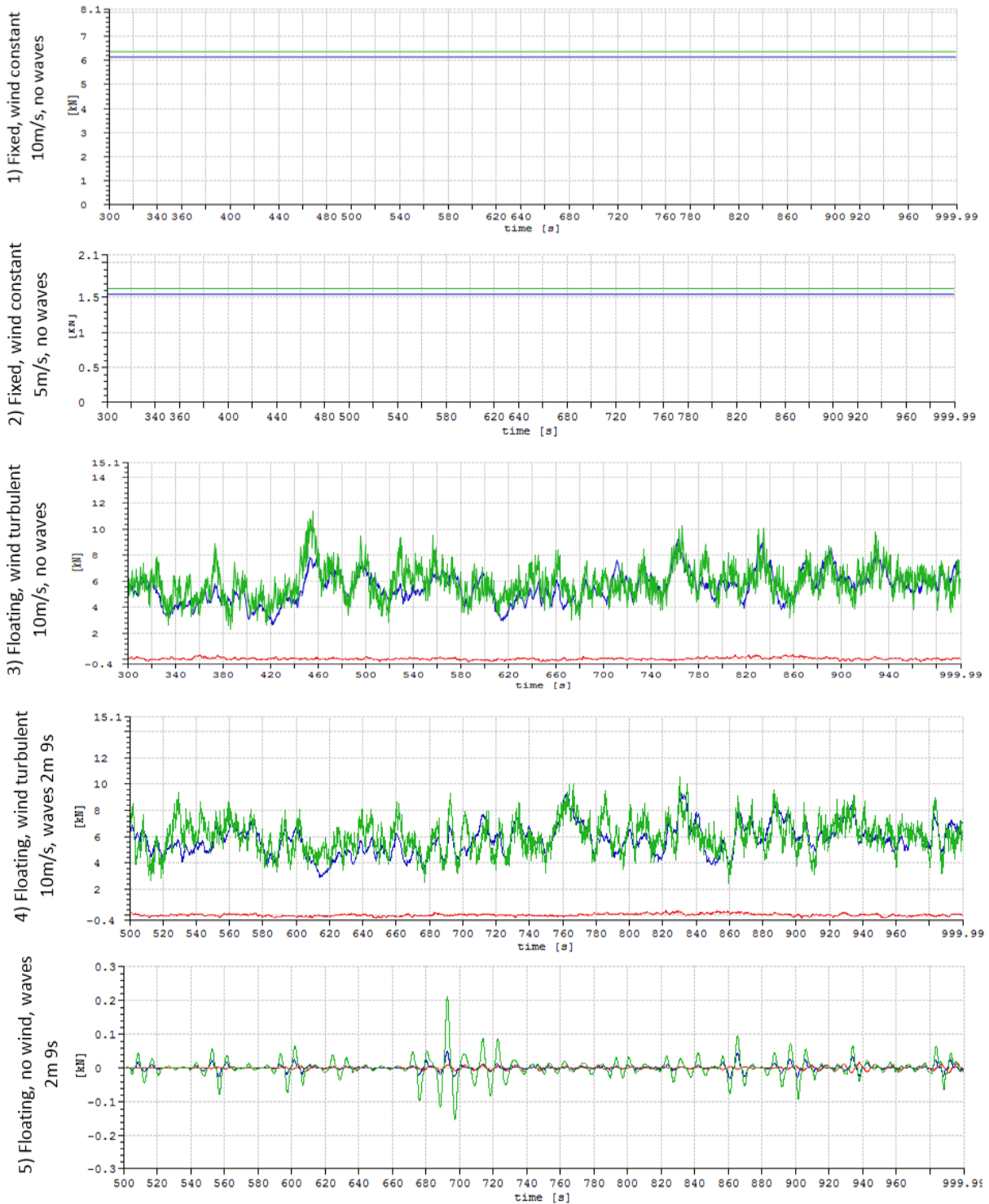
Figure C.1: Wind force acting on the B+F body for tests 1 to 5. X-component in blue, Y-component in red, Z-component in green
