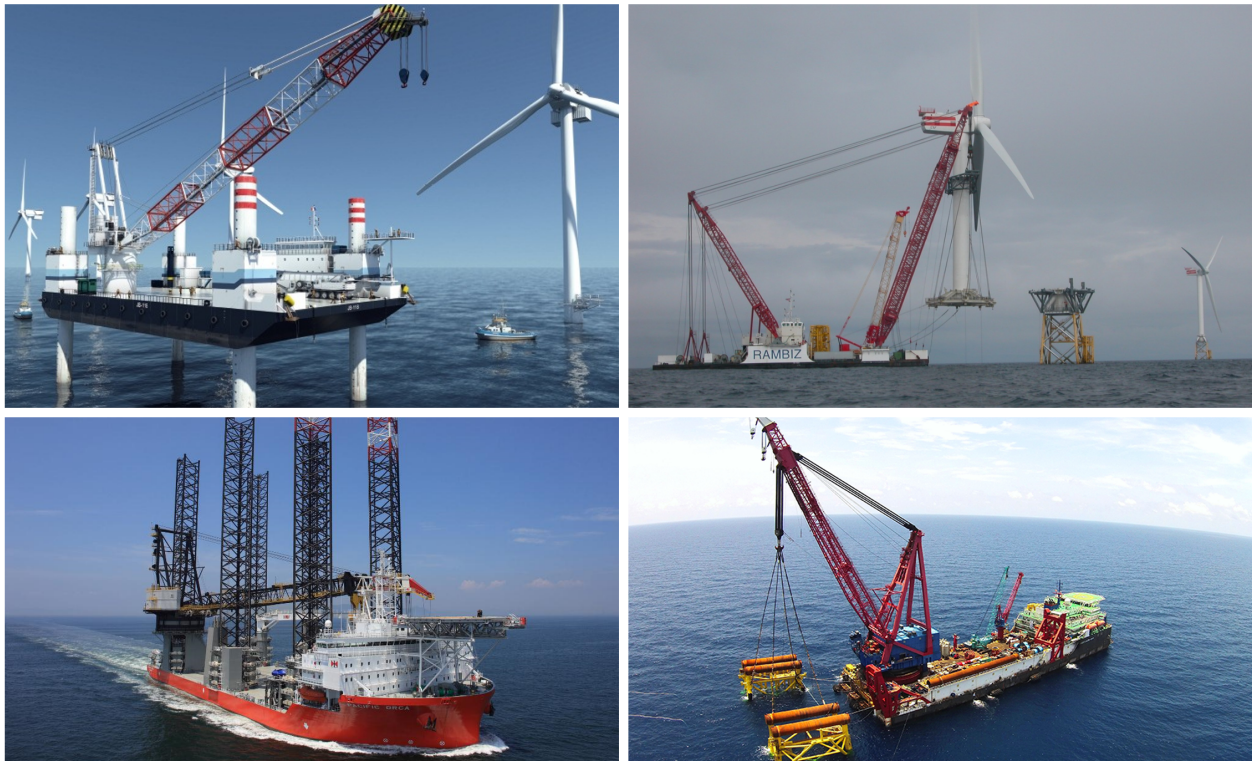
Figure 2.4: Vessels used for OWT installation. From top left, clockwise: Artist view of the Mir-Tac's Jack-up barge (Picture: offshorewind.biz), Crane barge (Picture: Scaldis), DP crane vessel Swiber Kaizen 4000 (Picture: thrustmaster.net) and Wind Turbine Installation Vessel Pacific Orca (Picture: worldmaritimeneews.com)
