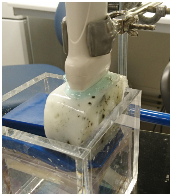
Figure 3.7: The finished heterogeneous phantom during measurements. The picture is taken a while after it was finished and had considerable bacterial growth.
