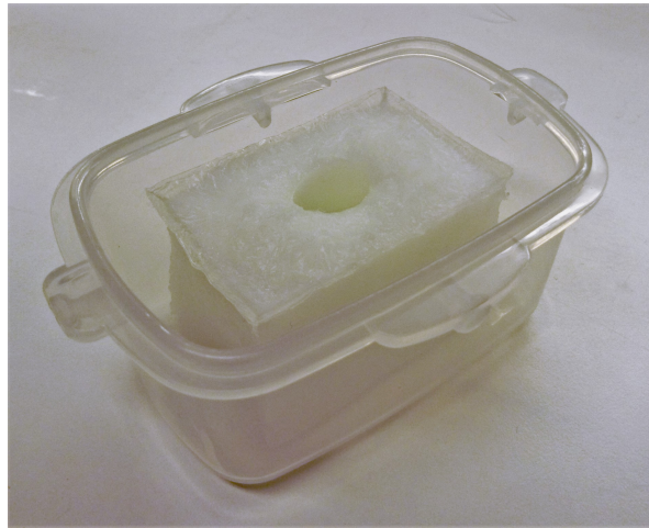
Figure 3.6: The second mold with the first rectangular PVA phantom, before adding more PVA mixture.
