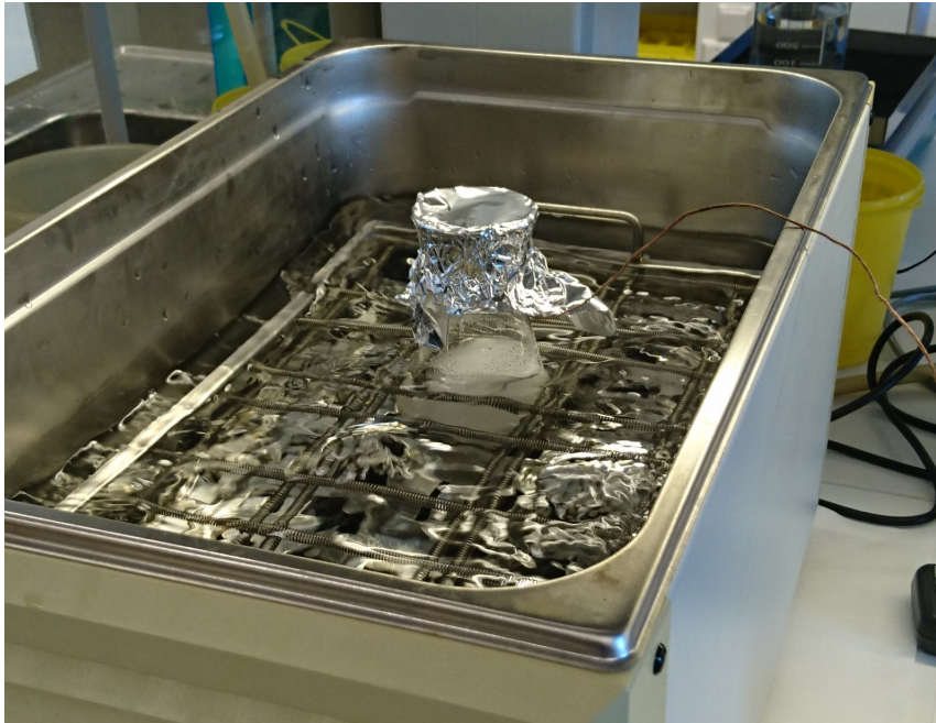
Figure 3.3: The PVA mixture in the water bath during the heating process. The bath was covered with a lid during this process.
