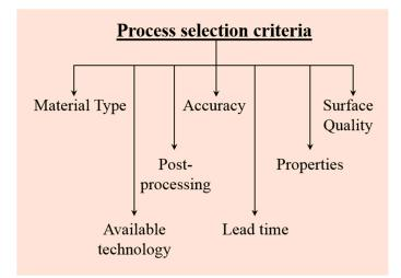
**Figure 1.** Schematic illustration showing the different factors that should be considered in selecting the right additive manufacturing process (binder jetting, selective laser melting, or electron beam melting).
