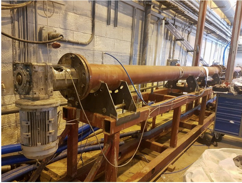
Figure 10 Test section with rotating drill string-motor
