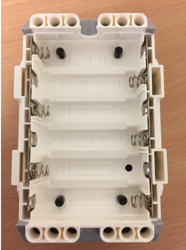
Figure 2.1: Removing the screws
