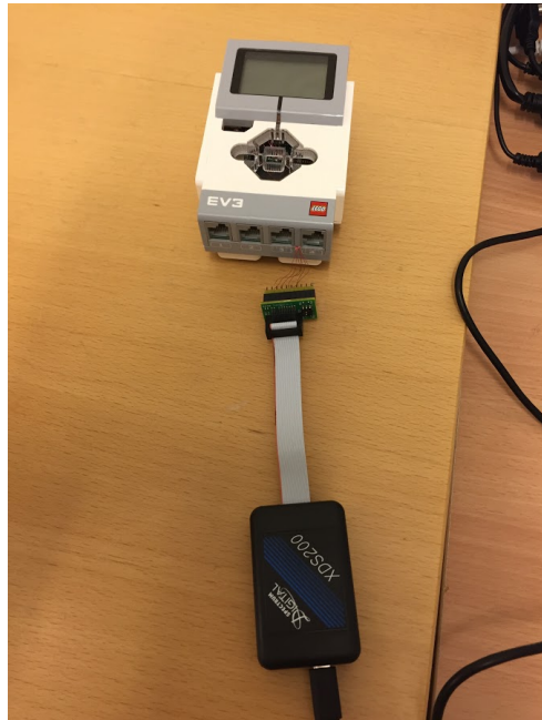
Figure 2.9: XDS200 connected to the Lego EV3.
