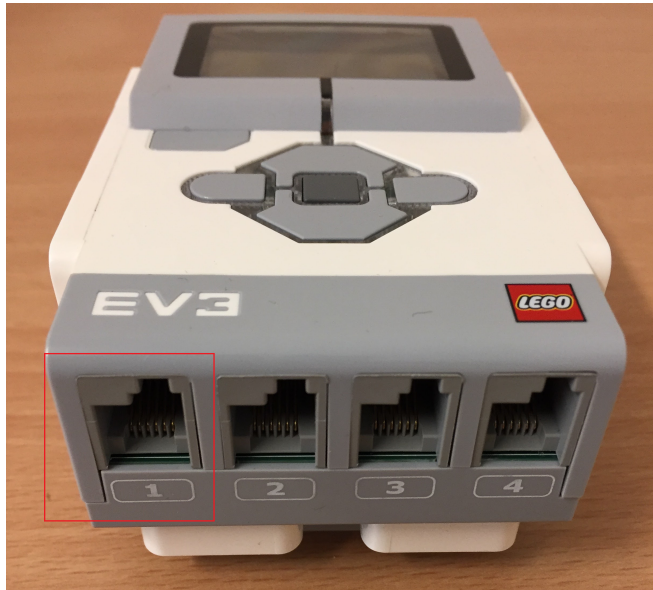
Figure 2.12: Port with interactive serial console interface
