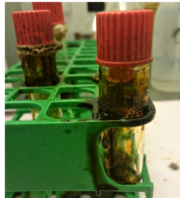
Figure 3.6: Attempted microwave assisted alkaline extraction of S. latissima , illustrating loss of product due to inappropriate vessels.
